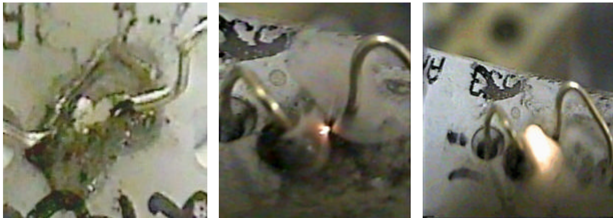
Figure 7. From left to right: silver layer forming at positively charged Ag wire (right wire), constant glow/smoke created by initial fuel drop and fuel vapor ignition by constant glow for terminal block experiments with “low sulfur” fuels and 40Vdc, 30 – 74 mA power supplies.
