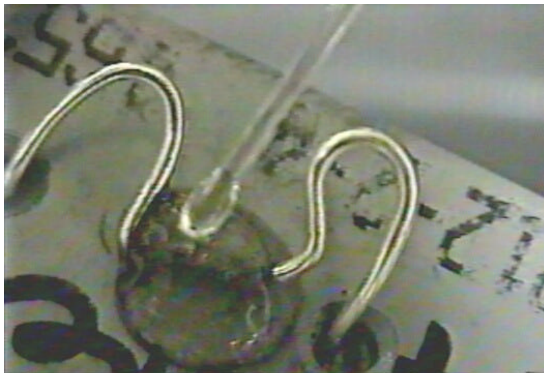
Figure 6. Pipetting fuel drop (5 microliters) onto water drop between two Ag wires on back of terminal block.
