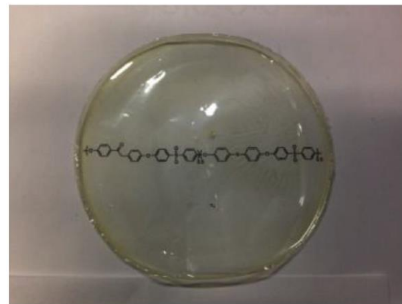
Solution cast film of deoxybenzoin-containing polysulfone
