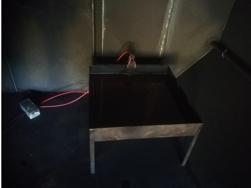
Figure 4 – Surface burning scenario arrangement
