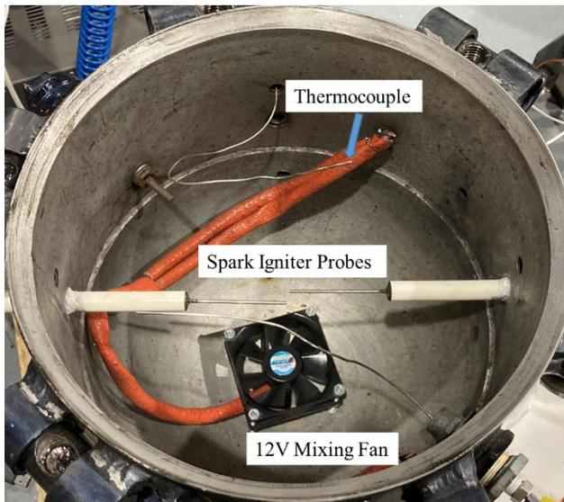
lithium battery thermal runaway. Simulations were also performed to predict the effectiveness of various extinguishing agents at elevated temperatures and decreased pressures.
