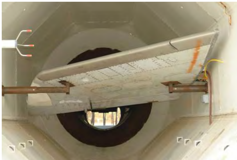
Figure 2. Wing Fuel Tank Test Article Installed in the Wind Tunnel
