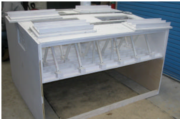
Figure 1: Scale A320 CWT Plywood Model
