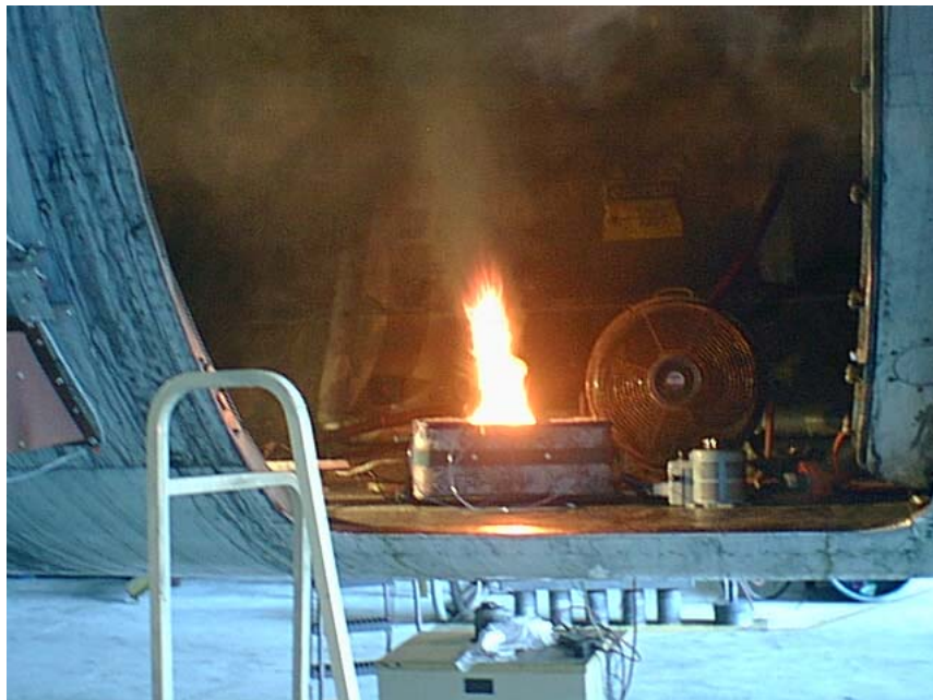
FIGURE 4. FULL-SCALE B-707 CARGO COMPARTMENT FACILITY
