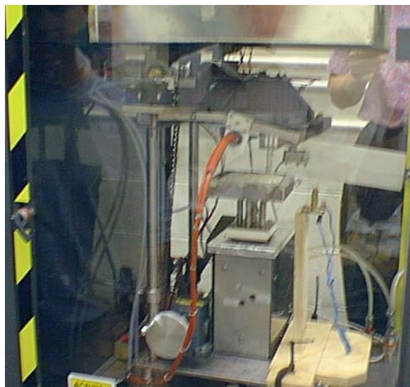
FIGURE 2. CONE CALORIMETER FACILITY
