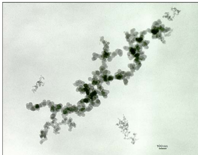
FIGURE 6. TRANSMISSION ELECTRON MICROSCOPY IMAGE OF SOOT AGGREGATES
