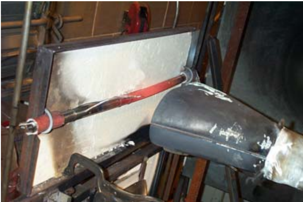
FIGURE 10. 15-5 PH STEEL BAR AFTER TEST
