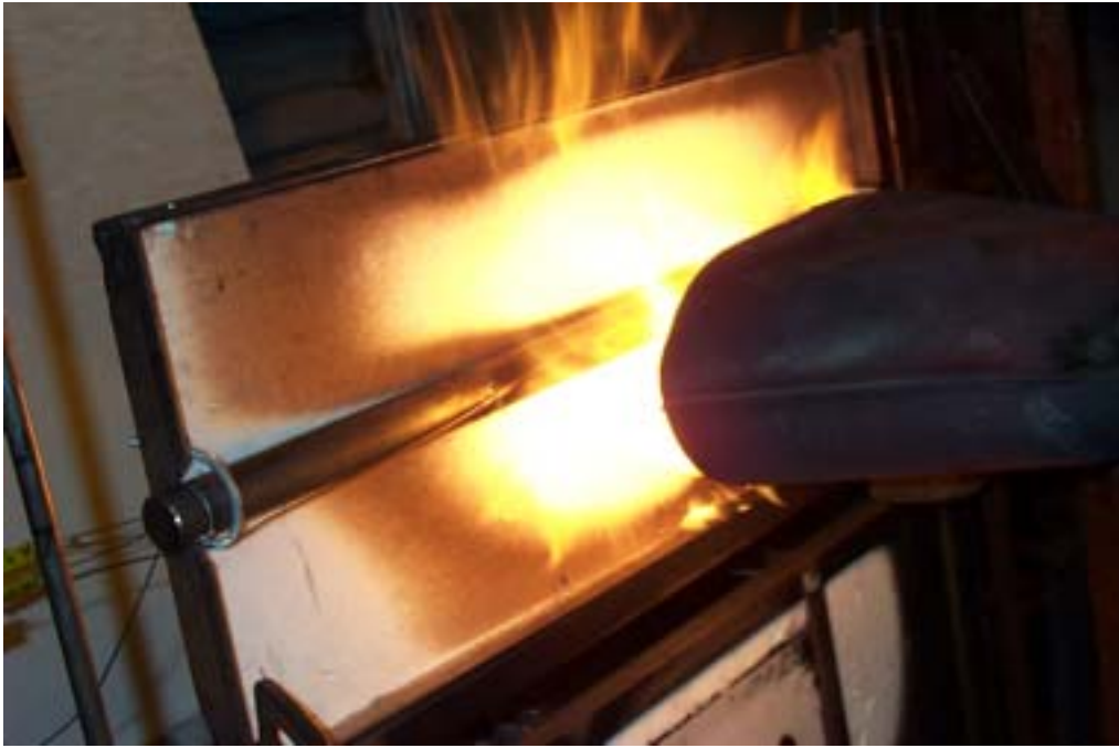
FIGURE 9. FIRE TEST OF 4130 STEEL BAR
