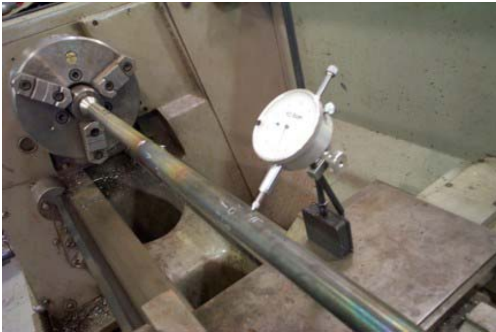
FIGURE 36. TEST FIXTURE DURING THE DETERMINATION OF THE SPECIMEN MAXIMUM DEFLECTION
