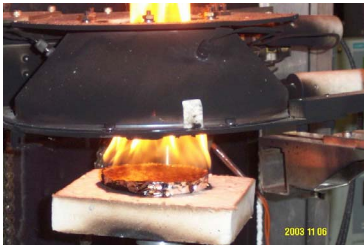
Figure 5. Liquid-like Steady Burning of 4-mm Nylon Under 56 \text{ kW/m}^2 Heat Flux
