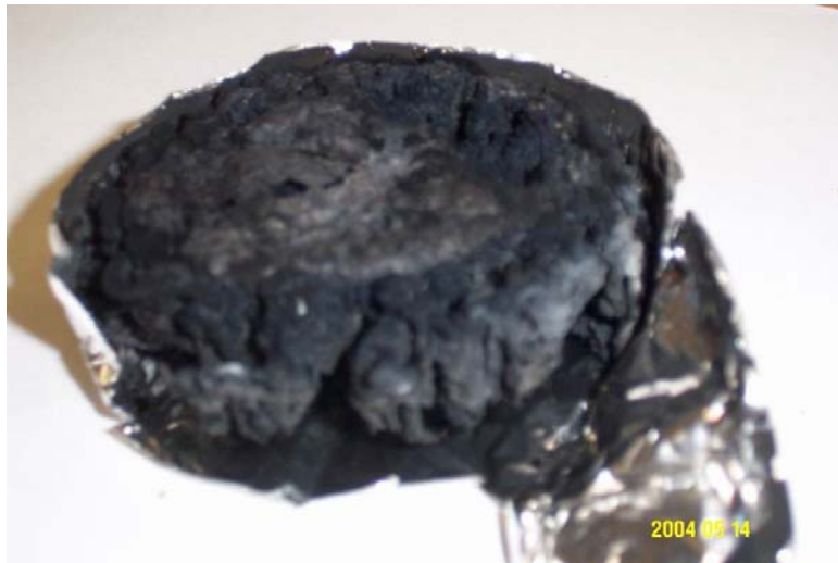
Figure 12. A 24-mm Nylon +5% Clay Under 50 kW/m 2 Residue After Burning
