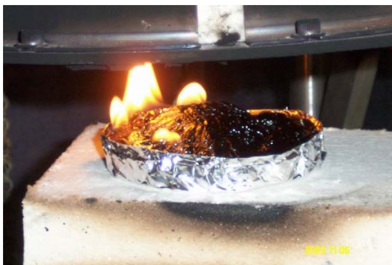
Figure 10. An 8-mm Nylon +2% Clay Test Sample Under a 34 \text{ kW/m}^2 Heat Flux Burning at Leaks at the Edge
