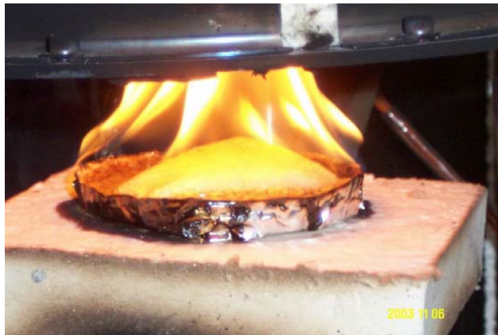
Figure 4. A Burning 4-mm Nylon Center Rising Due to Swelling Under 56 \text{ kW/m}^2 Heat Flux
