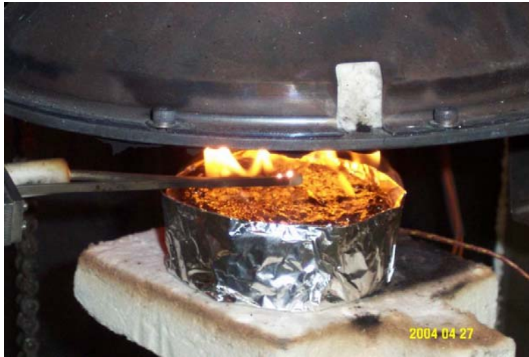
Figure 8. A Test Sample of 24-mm Nylon + 2% Clay Just After Ignition Burning Under 50 \text{ kW/m}^2 Heat Flux
