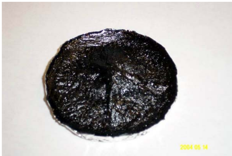
Figure 7. A 3.2-mm Nylon Sample at 16 kW/m 2 Heat Flux With no Ignition, but Oxidized and formed a Carbonaceous Skin
