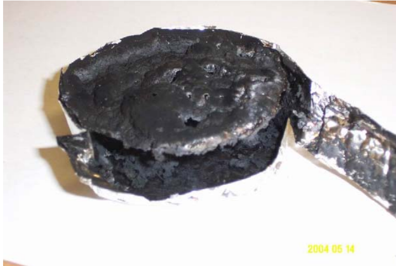
Figure 11. A 24-mm Nylon +2% Clay Test Sample Under 50 kW/m 2 Residue After Burning
