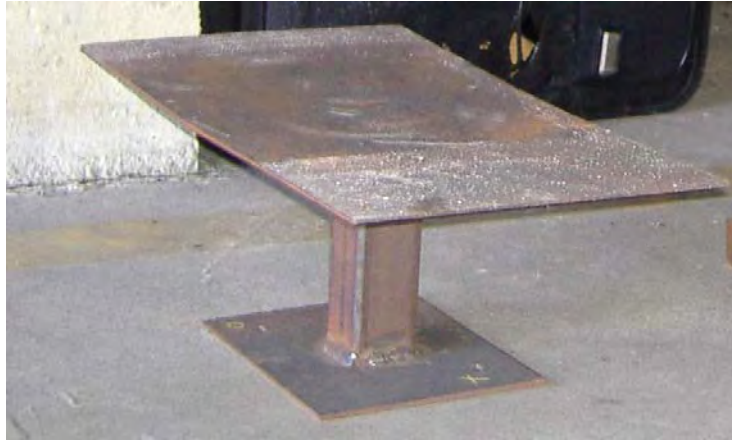
Figure 15. Extension Stand Welded for Vaporizer and Arizona Test Dust Tests
