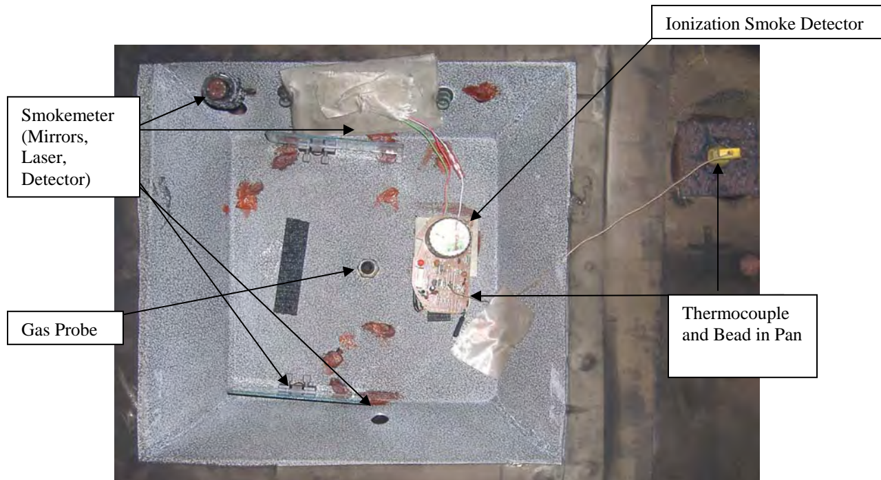
Figure 3. Recessed Pan Including All Sensor Instrumentation
