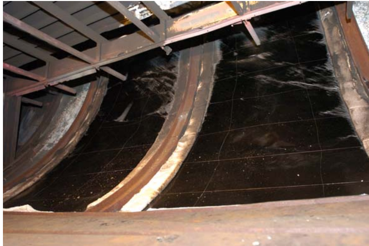
Figure 60. Posttest Inspection of the Inboard Surface of the Carbon/Epoxy Structural Composite Material
