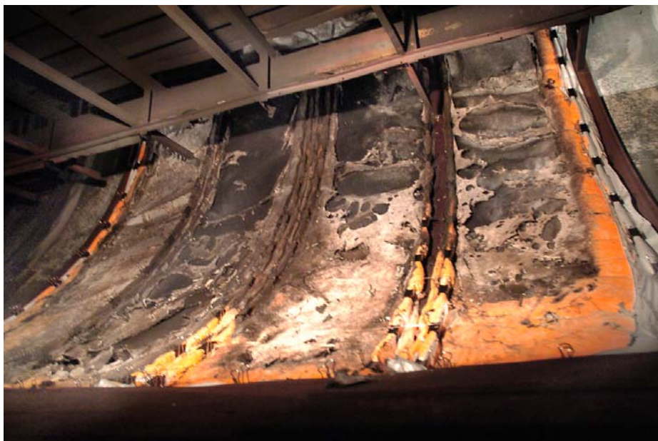
Figure 52. Posttest Inspection of Inboard Side of the Fiberglass/Ceramic Barrier Insulation System
