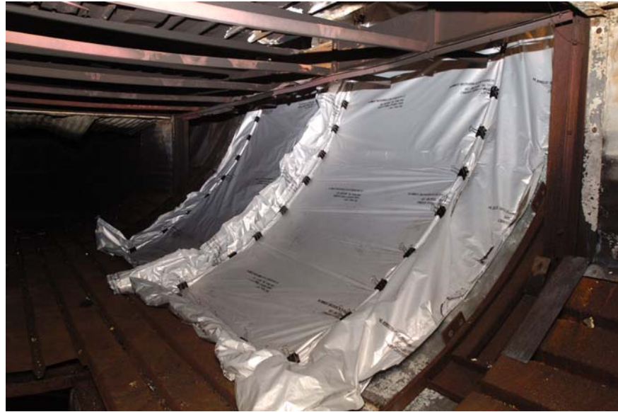
Figure 37. Full-Scale Test Apparatus Showing Typical Clipping Arrangement of Insulation Blankets
