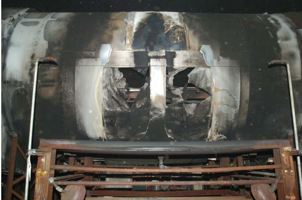
Figure 49. Posttest Inspection Shows Failure of the Ceramic Barrier During Initial Configuration
