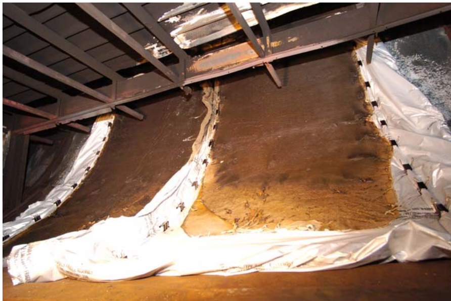
Figure 40. Posttest Inspection of PAN Material, Shown From Inboard Side
