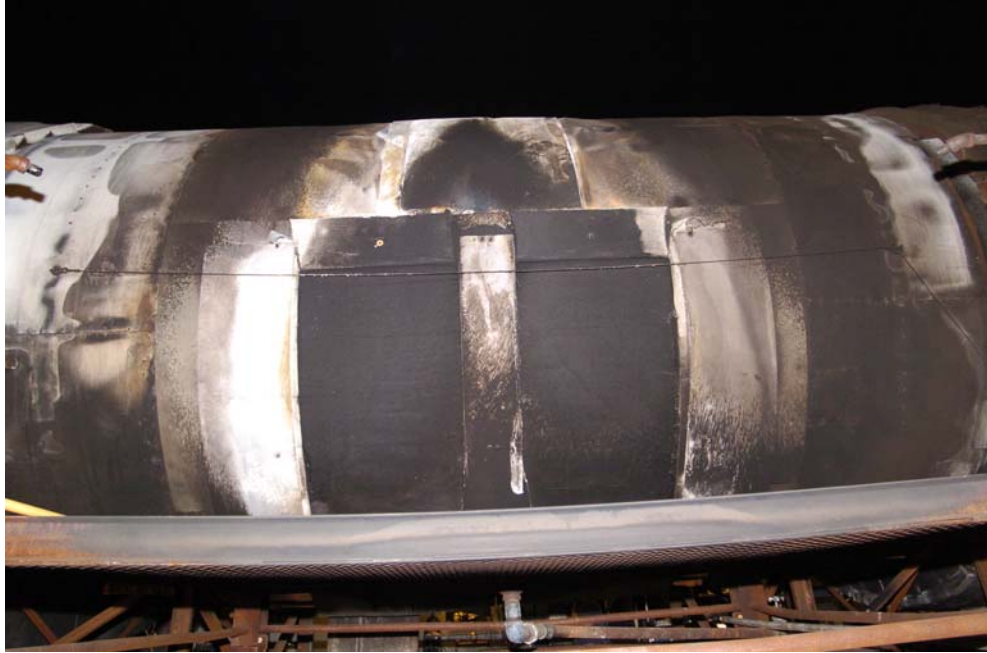
Figure 41. Posttest Inspection of PAN Material, Shown From External Side
