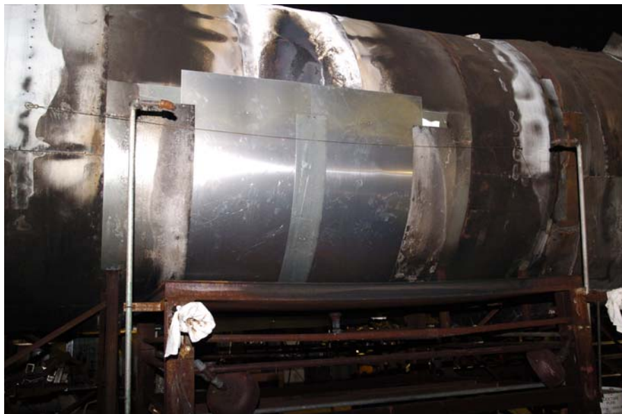
Figure 38. External Face of the Full-Scale Test Apparatus Showing Aluminum Skin
