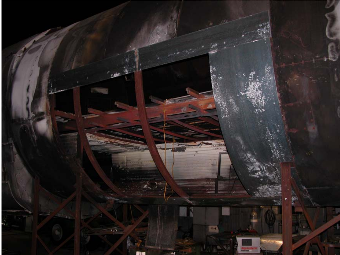
Figure 35. Full-Scale Test Apparatus Configuration for Evaluating Decomposition Products From Various Insulation Samples
