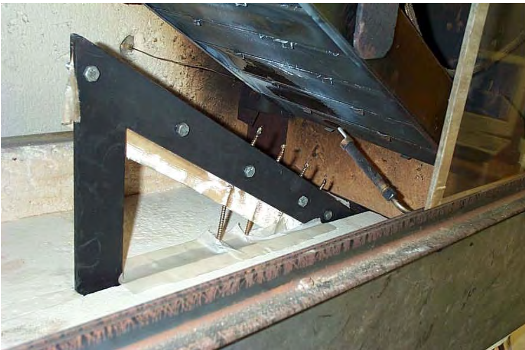
Figure 6. Thermocouples Characterization Fixture Inside RHP Apparatus
