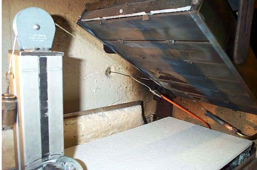
Figure 13. Short Wire Mounted on the Sample Holder Using Alligator Clips
