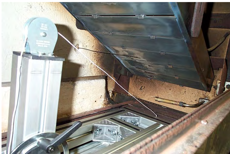
Figure 11. Wire Mounted on the Sample Holder at a 30-Degree Angle
