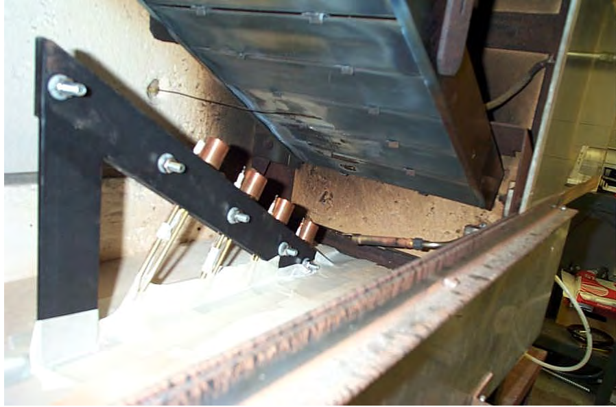
Figure 7. Calorimeter Characterization Fixture Inside RHP Apparatus
