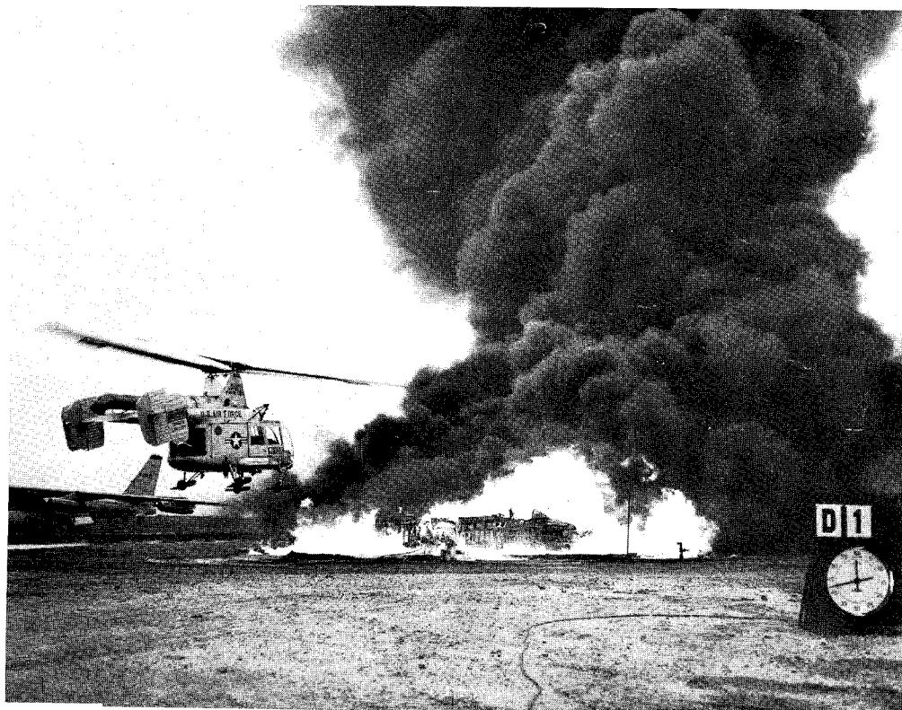
(b) FIRE CONFIGURATION 12 SECONDS AFTER THE START OF FOAM DISCHARGE
