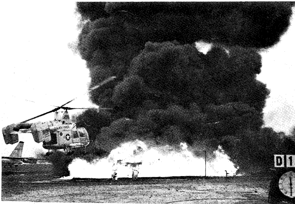
(a) FIRE CONFIGURATION 1 SECOND BEFORE THE START OF FOAM DISCHARGE
