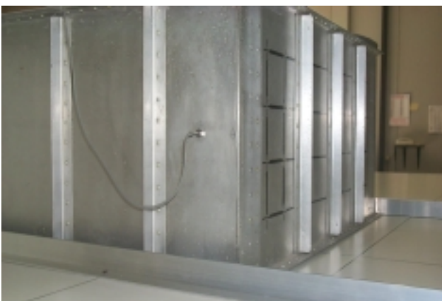
Fig. 6 - Test equipment: right side pressure transducer.
