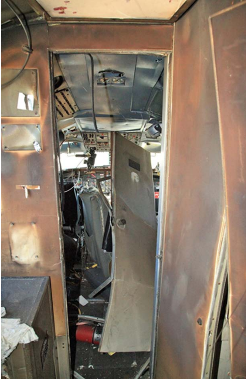
Figure 21. Flight deck bulkhead damage and door
