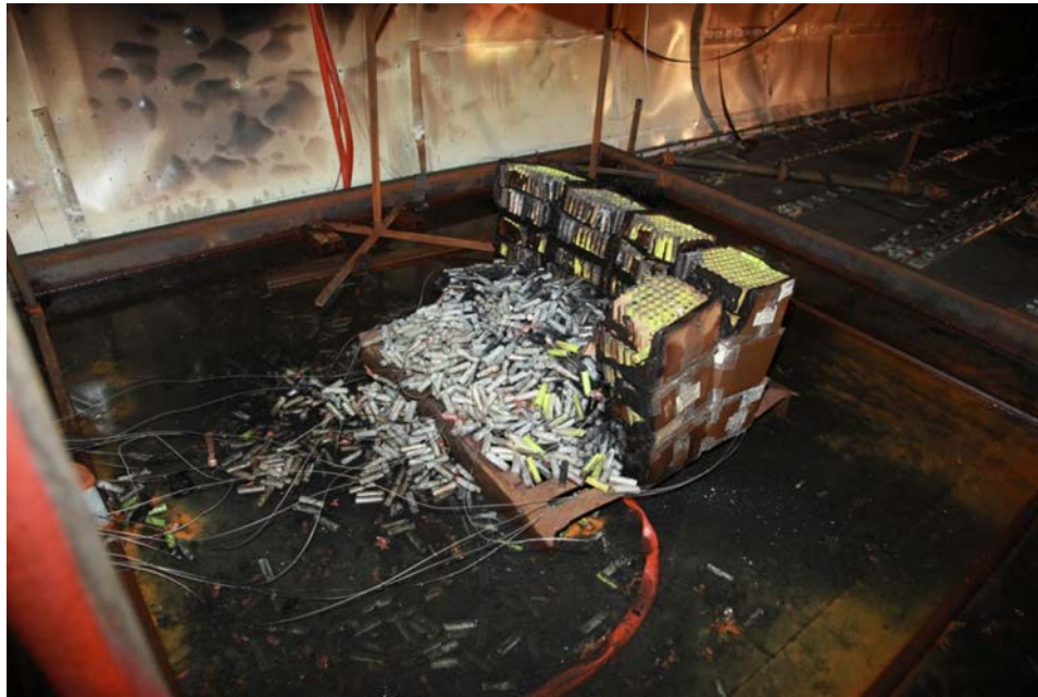
Figure 15. Lithium-ion cells consumed post test
