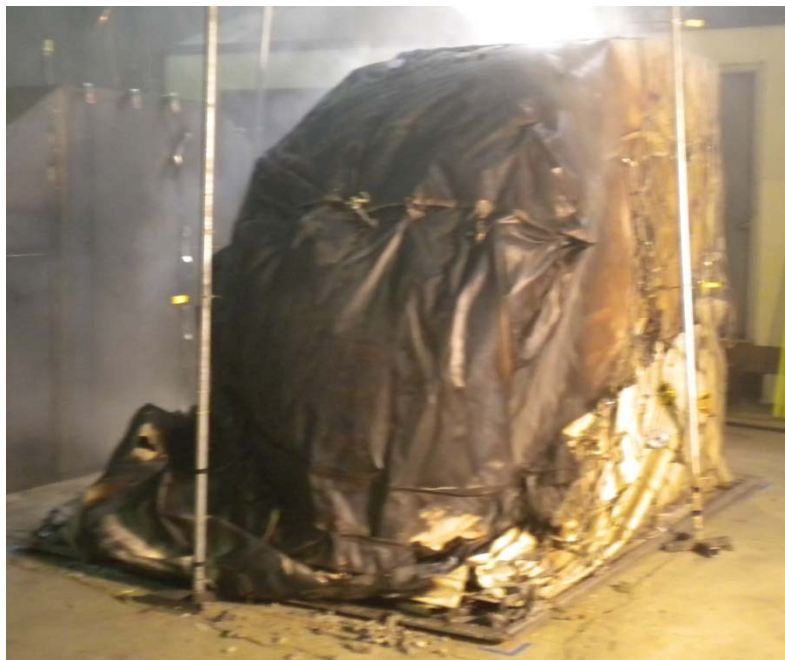
Figure 26. Full-scale fire test of an FCC
