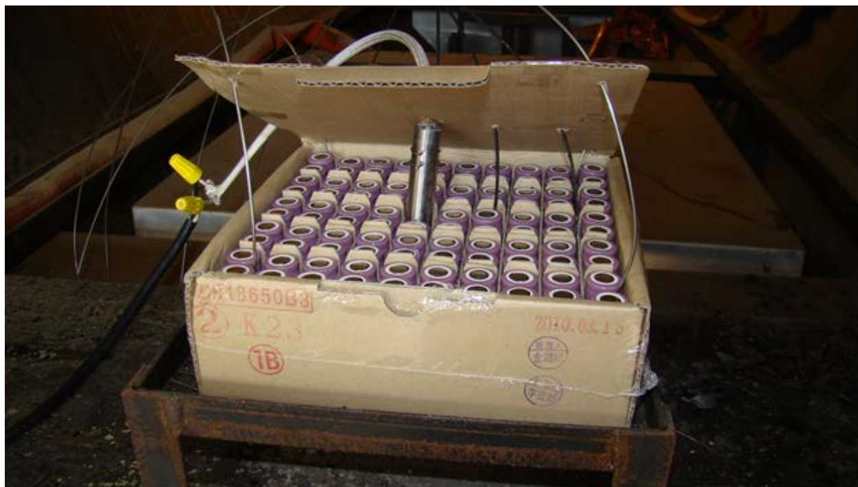
Figure 3. Shipping box with interlocking cardboard separators for 100 18650 LiCoO 2 lithium-ion cells
