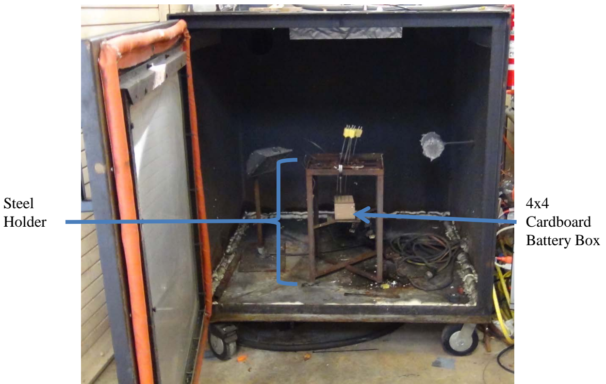
Figure 47. Test chamber and setup
