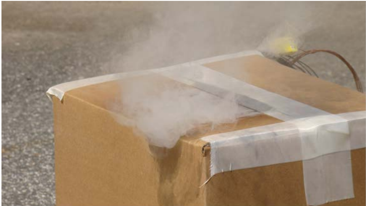
Figure 6. Oxygen-generator overpack test
