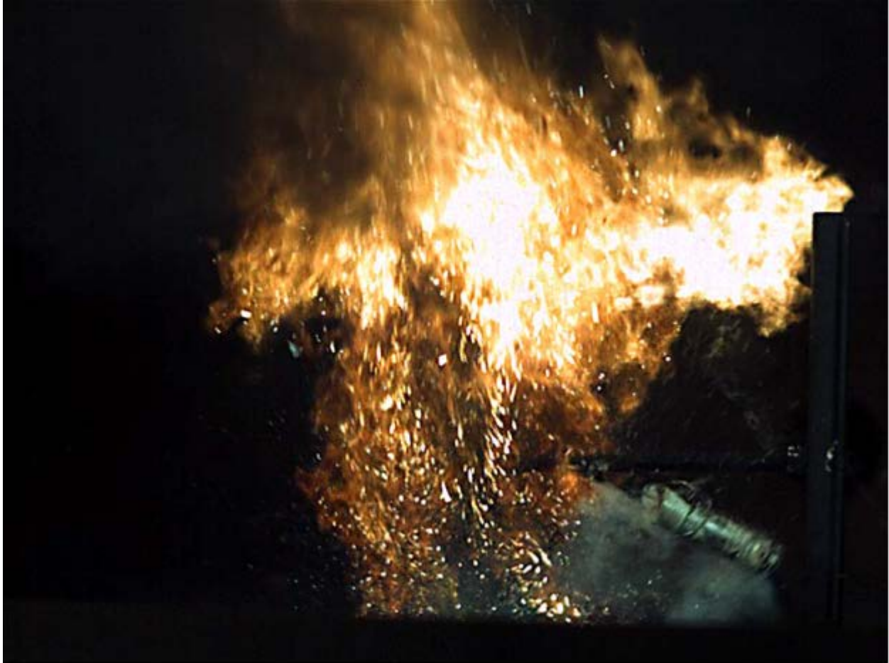
Figure 2. High-speed video capture of a lithium-ion LiCoO 2 cell in catastrophic disassembly
