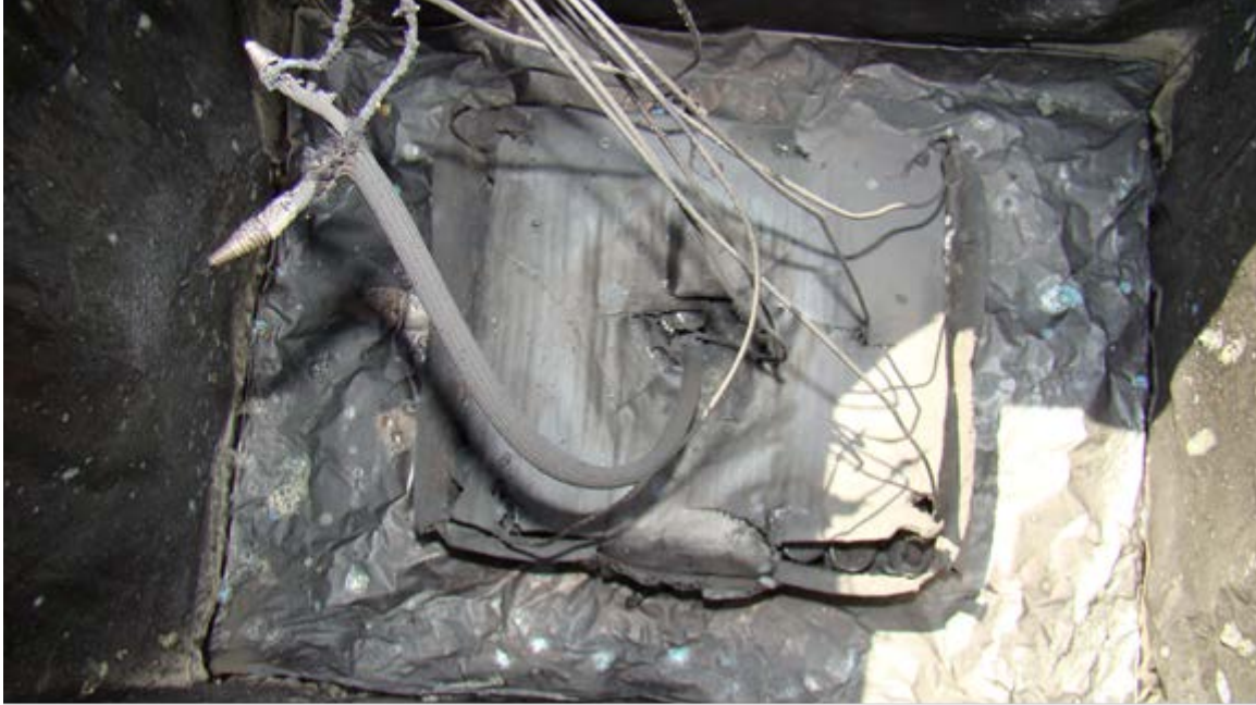
Figure 7. Oxygen-generator overpack post test
