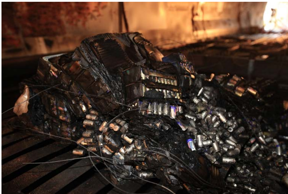
Figure 16. Lithium-metal cells post test
