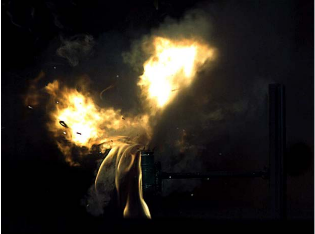
Figure 1. High-speed video capture of lithium-ion \text{LiCoO}_2 cell in thermal runaway
