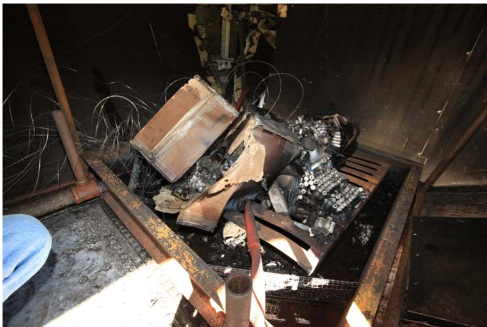
Figure 19. Lithium-metal cells post test
