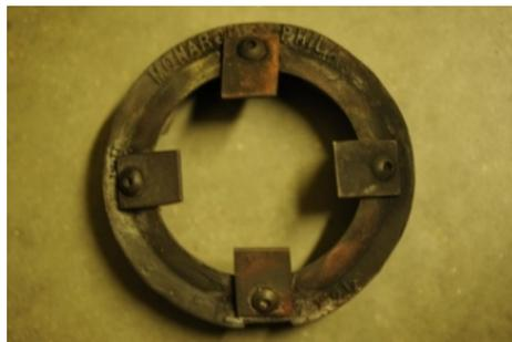
**Figure 4. Modified turbulator**
