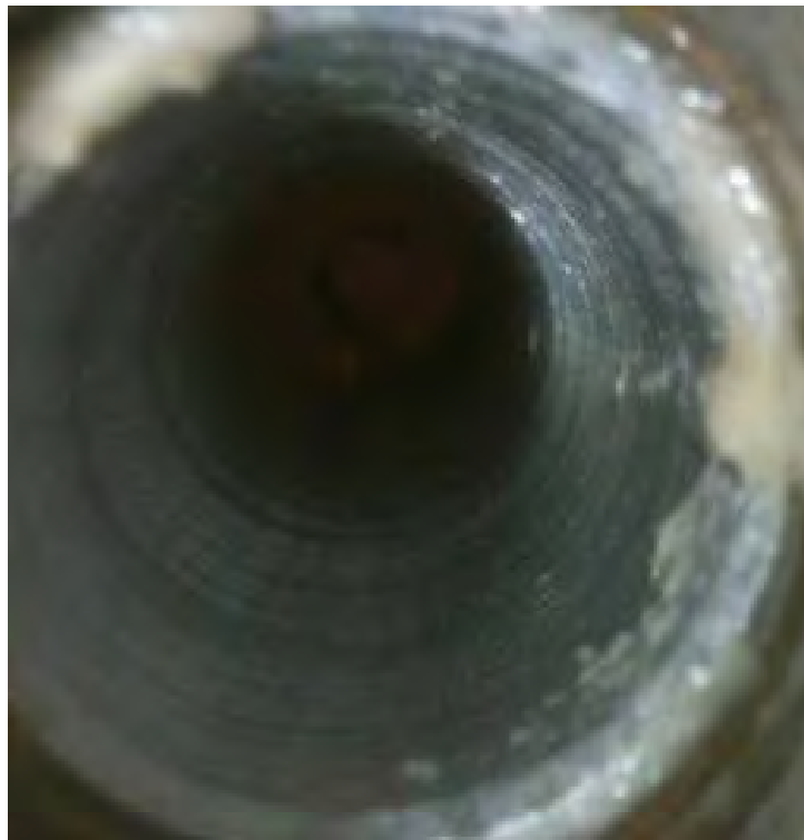
(b) Scratched Aluminum (Top Pipe)
