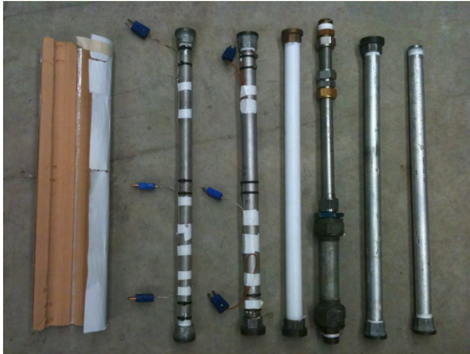
Figure 2.4: Insulation and Test Pipes. From Left to Right: Polyurethane Insulation, 3/4" Stainless Steel, 1" Stainless Steel, 1" Teflon, 1"/1.5" Area Change, Scratched Aluminum, Aluminum
