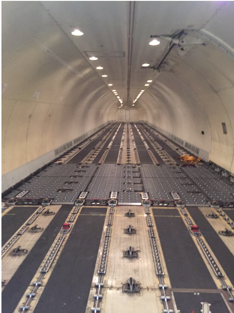
Figure 1.5: Example of a cargo compartment space (Class E).
