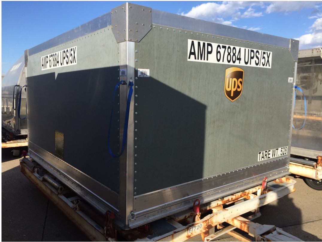
Figure 1.6: Example of a ULD.
