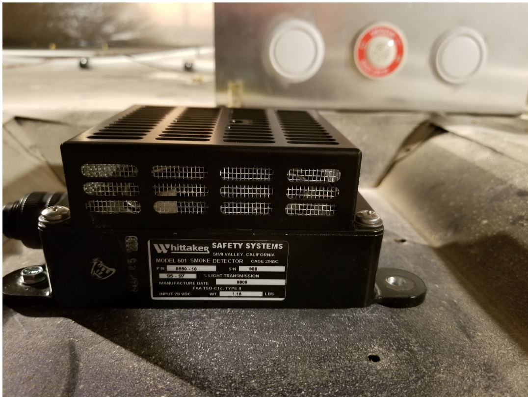
Figure A.9: Whittaker photoelectric spot detector.
