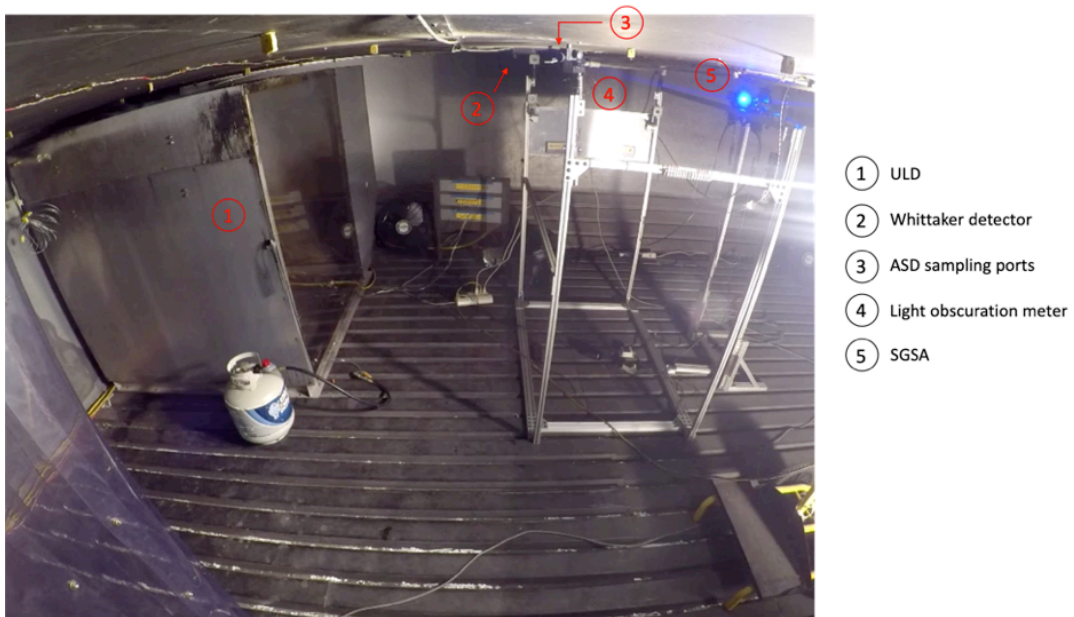
Figure A.8: Photo from FAATC ULD in cargo compartment testing.
