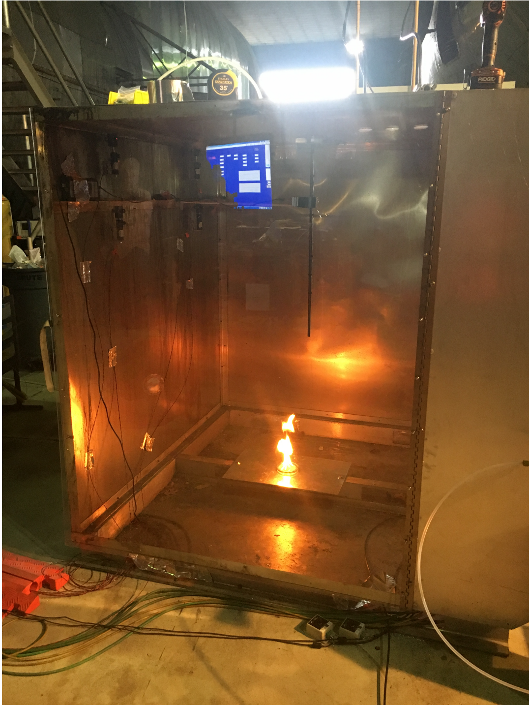
Figure A.5: Photo from FAATC ULD heptane test.
