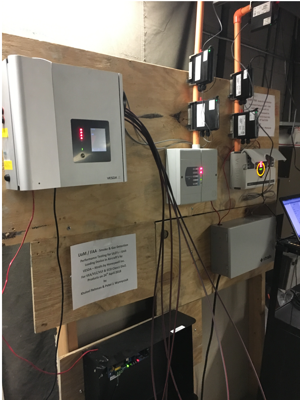
Figure A.3: Close-up of ASD setup at UMD.
