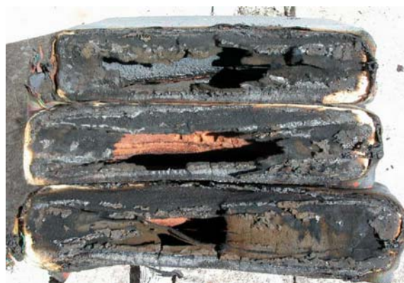
Figure 5. Fire-Blocking Layer; Horizontal Cushions
