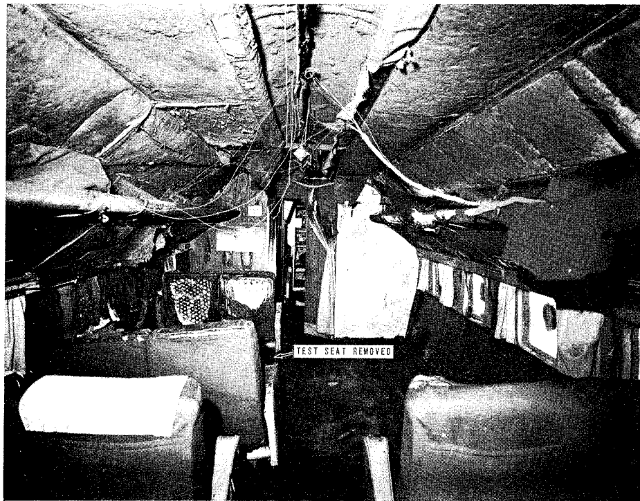
TEST NO. 41 AFTER FIRE
