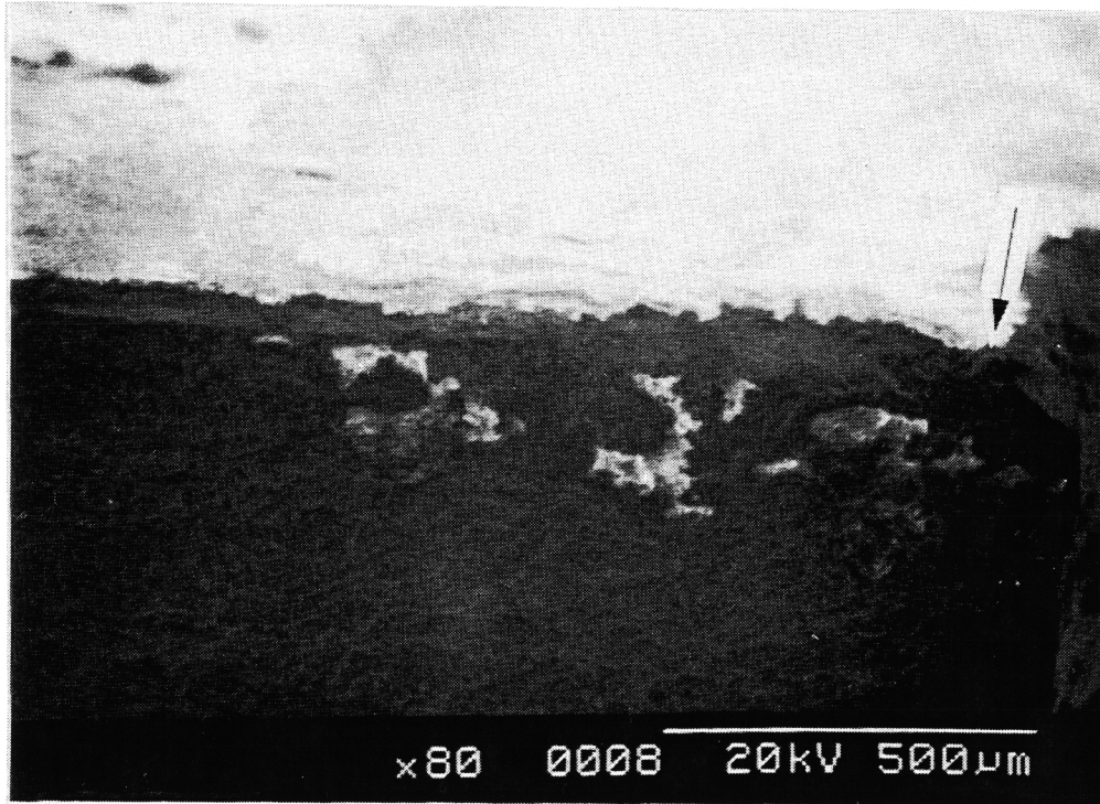
Figure 29. Fracture surface (bottom of picture) for crack from a fretted area (see arrow) between the plates. The substance at the top of the picture is interfacial sealant.
