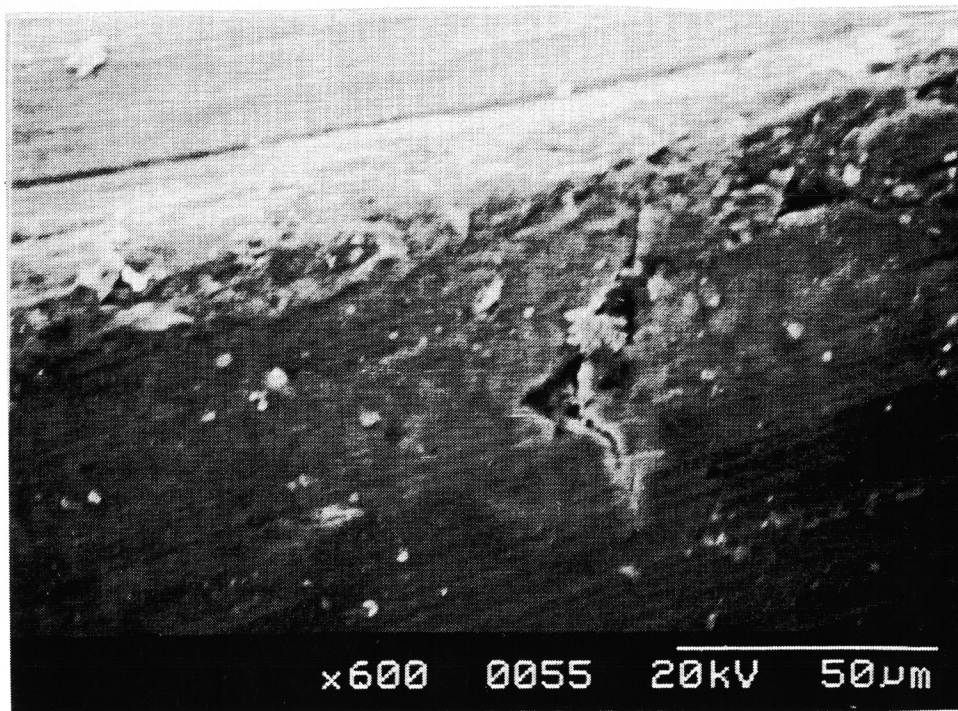
Figure 20. Crack emanating from a void or inclusion in a relatively unfretted region in rivet hole 49.
