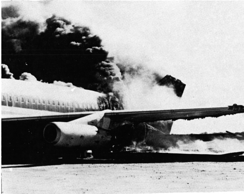
FIGURE 8. INTERNAL FIRE PROGRESSES FORWARD TO STATION 933, 10 MINUTES AFTER IGNITION
