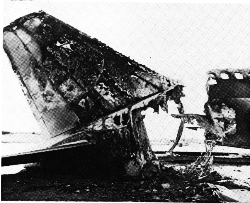
FIGURE 16. STARBOARD SIDE OF VERTICAL STABILIZER HEAVILY COATED WITH SOOT
