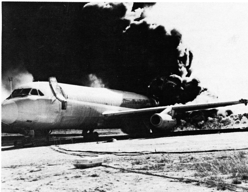
FIGURE 2. FLAME IMPINGEMENT ON PORT AFT FUSELAGE
