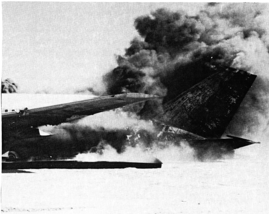
FIGURE 7. TAIL SEPARATES FROM FUSELAGE, 8 MINUTES 12 SECONDS AFTER IGNITION
