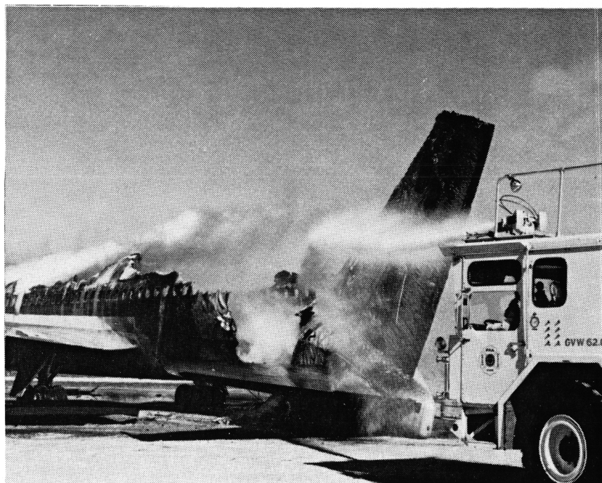
FIGURE 11. REMAINING FIRE IS EXTINGUISHED BY AIRPORT FIRE SERVICE, 33 MINUTES AFTER IGNITION
