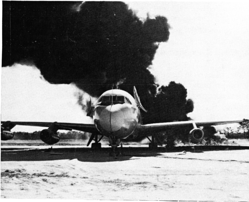
FIGURE 4. FULLY DEVELOPED FUEL FIRE, FORWARD VIEW, 20 SECONDS AFTER IGNITION
