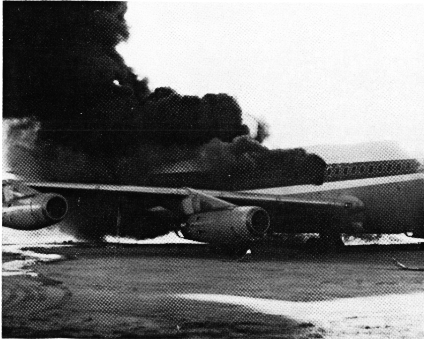
FIGURE 6. SMOKE POURS FROM STARBOARD OVERWING EXIT, 3 MINUTES 35 SECONDS AFTER IGNITION
