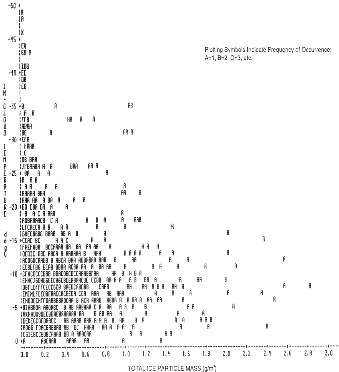
FIGURE 5c. COMPUTED, EVENT-AVERAGED, TOTAL ICE PARTICLE MASS VERSUS TEMPERATURE FOR ALL TYPES OF ICE PARTICLE CLOUDS
