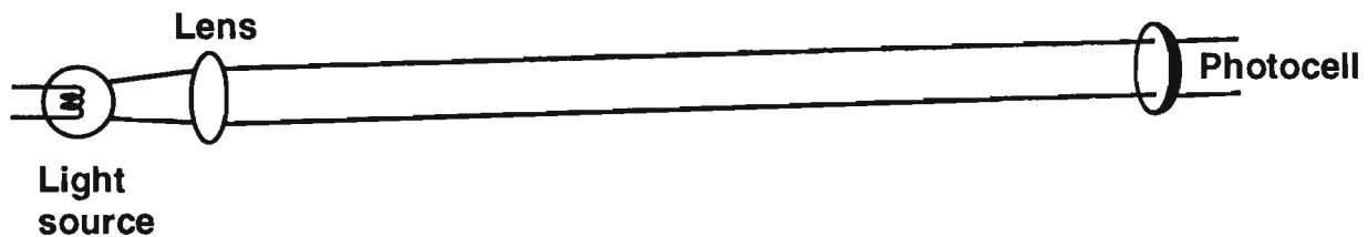
Figure 2-7. Light Attenuation Type Photoelectric Smoke Detector.
