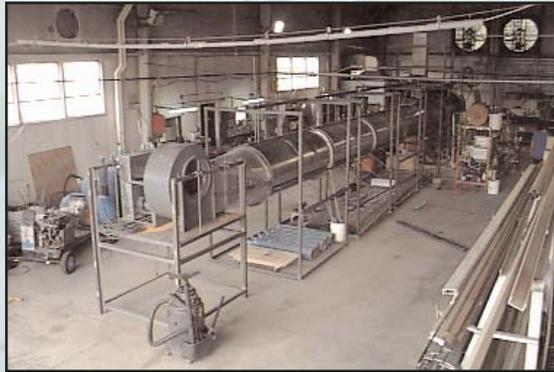
The Engine Nacelle Simulator will evaluate materials and technologies being considered as a halon replacement within the engine and APU compartments. By using a simulator and not a true aircraft engine for the bulk of the halon replacement work, maintenance costs will be reduced. Additionally, the generic geometry of the simulator can be used to develop a better understanding of the fire suppression environment.
