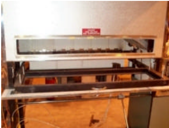
Fig: Radiant Panel Test Showing Sample Emplacement and Fueled Panel.
