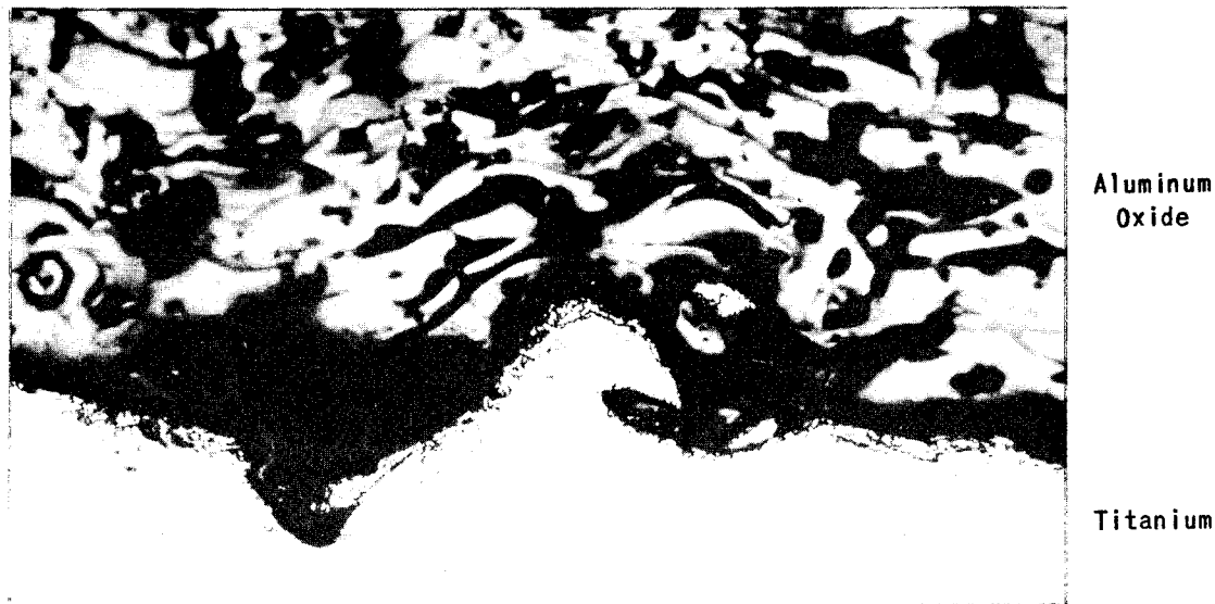
Figure 5. FLAME-SPRAYED ALUMINUM OXIDE ON TITANIUM
