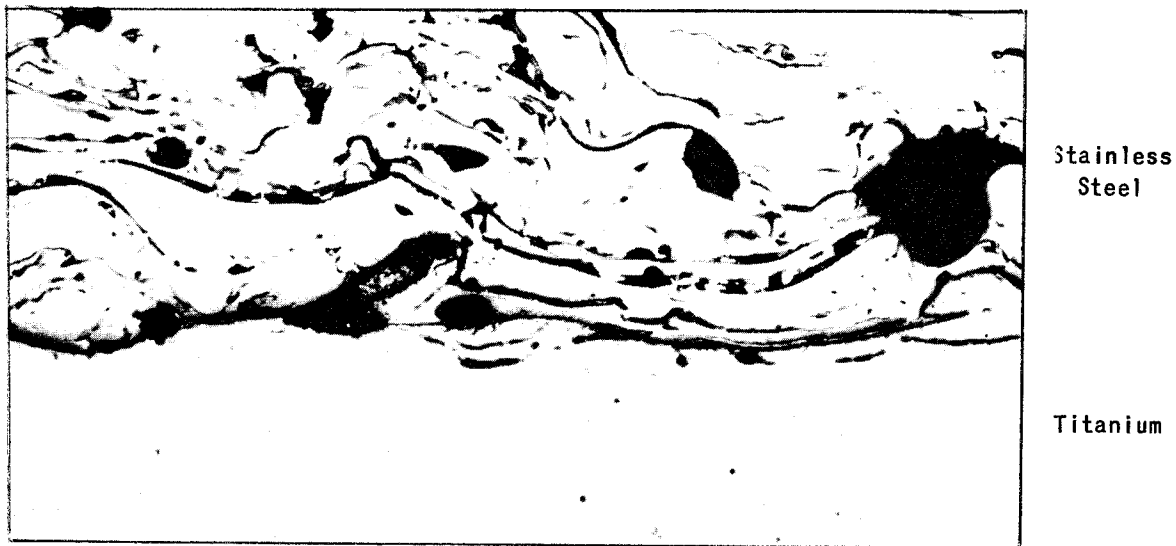
Figure 1. TYPICAL BOND BETWEEN FLAME-SPRAYED COATING AND METALLIC SUBSTRATE
