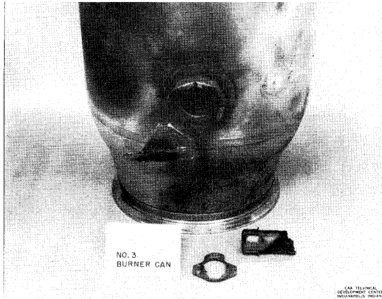
Fig. 29 Damage to Burner Can From Ingesting Sprayed Fuel into the Air Inlet of a J35-A-13D Engine While Operating at a Throttle Setting of 100 Per Cent (7,759 rpm)
