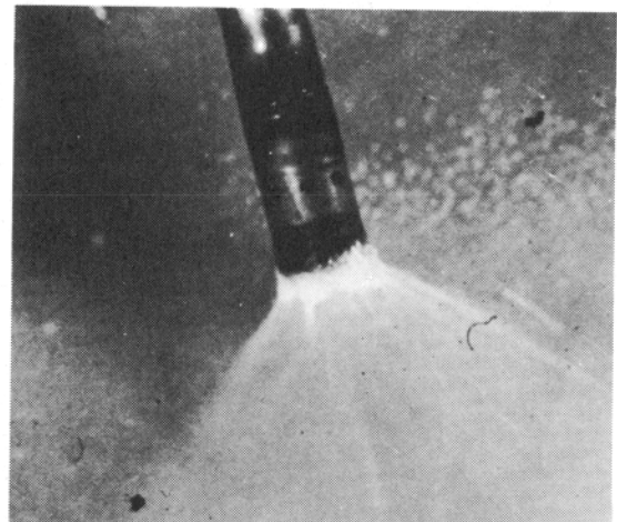
Fig. 8 - Emulsified fuel spray pattern, showing "globbing" at tip
