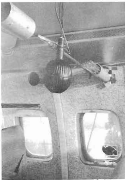
(d) Instrumentation for Full-Scale Flammability Tests—Shielded Thermocouples, Gas Sampling Tubes, Movie Camera Outside
