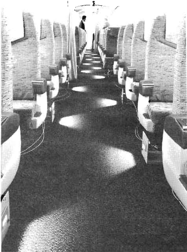
(d) Underseat Aisle Lighting Concept (One of three aisle lighting concepts tested, using individual test subjects in evaluating 11 test conditions of aisle light level and uniformity)
