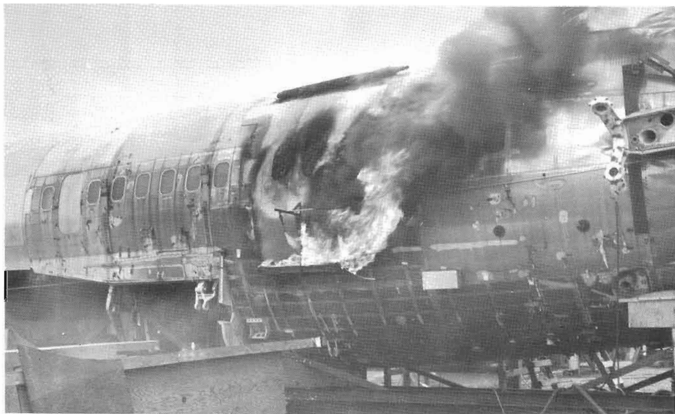
(a) External Fuel Fire -6.25-Sq-Ft Fuel Pan for Flammability Test of Interior Materials
