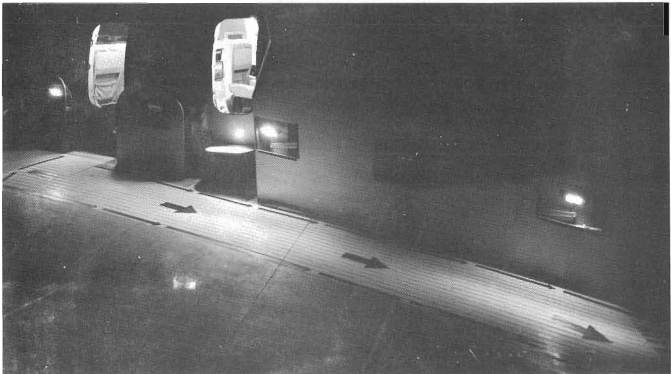
(c) Experimental Uniform Lighting—0.1 ft-c Average Illumination on Entire High-Reflectance Overwing Path
