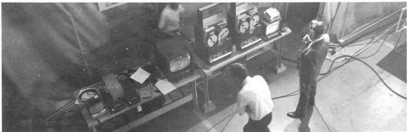
(f) Infrared Television Monitor and Tape Recorders Set Up Outside Lightproof Tent
