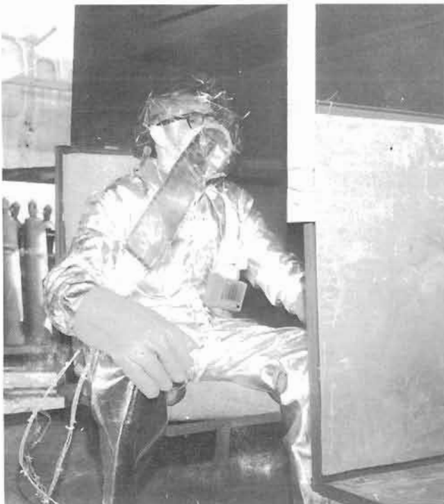
(g) Smoke-Hood Test Subject in Position for Exposure to Jet-Fuel Fire
