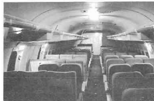
UNIFORMITY OF ILLUMINATION CONTROLLED (0.1 ft-c AVERAGE, 0.01 ft-c MINIMUM)
