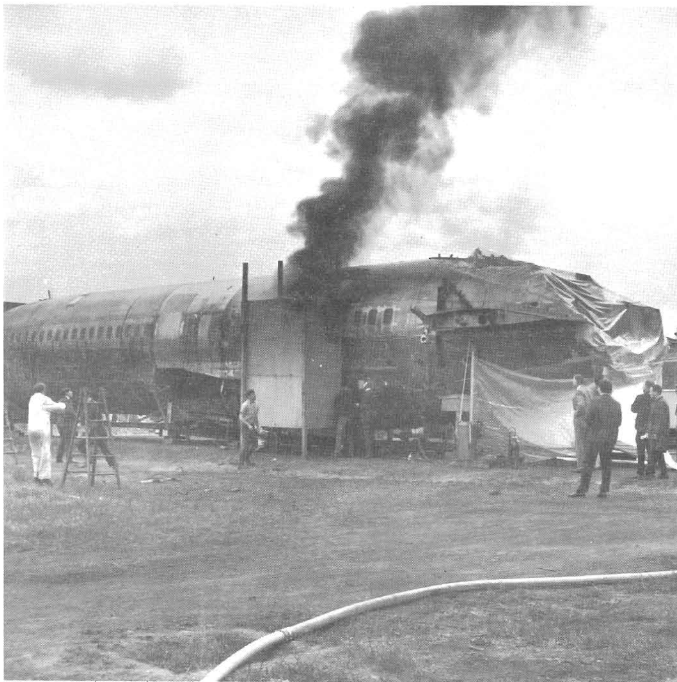
(a) Full-Scale Fire Test Fuselage Section—Windshield in Place Around Fuel Pan Next to Fuselage Rupture for Furnished Interior Materials Test
