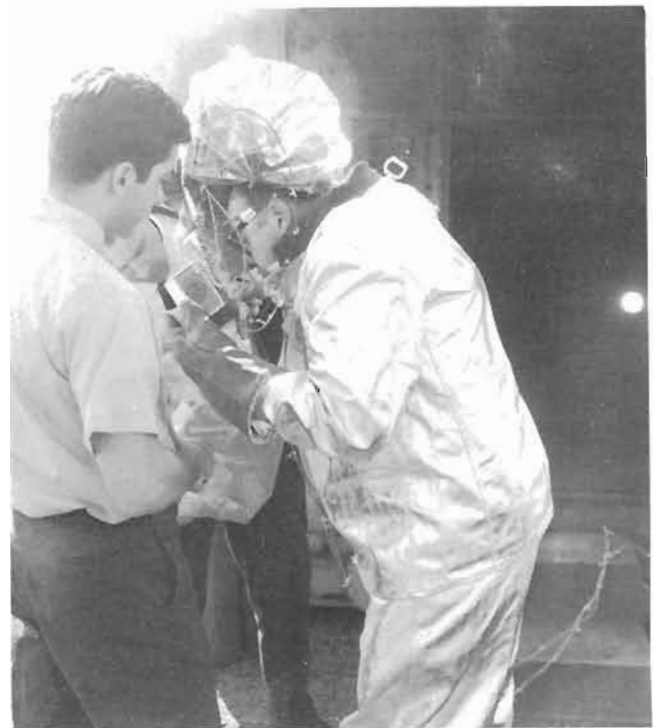
(h) Breath Sample Being Taken after Exposure of Smoke- Hood Test Subject to Jet-Fuel Fire
