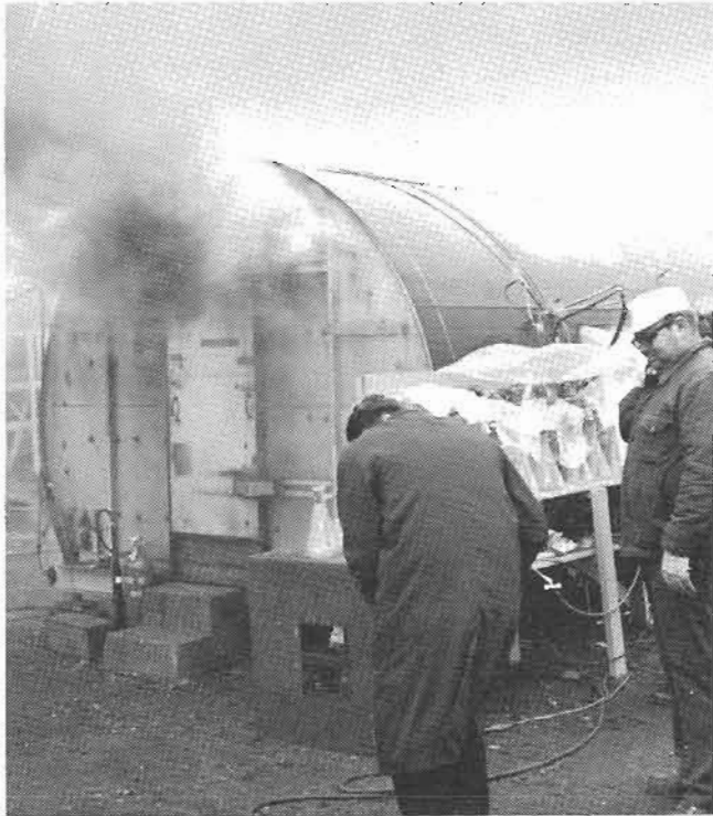
(f) Short Fuselage Section for Materials, Suppression, and Smoke-Hood Tests
