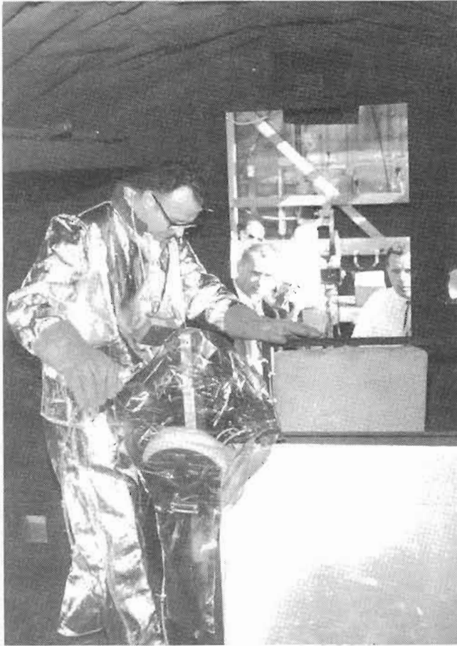
(b) Smoke-Hood Testing In Jet-Fuel Fire Environment
