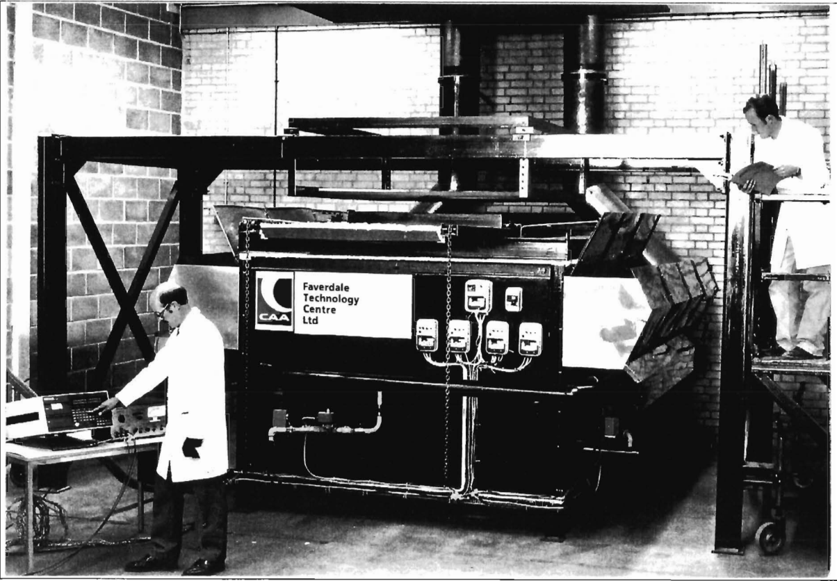
The fuselage burnthrough facility at Faverdale Technology Centre, England
