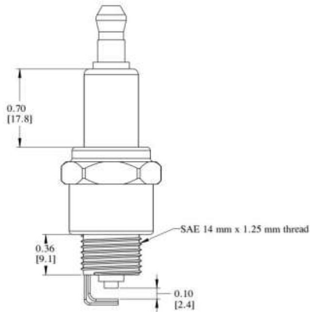
Figure 25-32. Dimensioned Drawing of a Spark Plug
