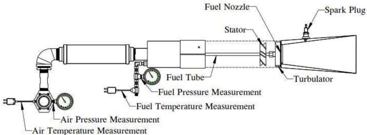
Figure 25-5 Inlet Condition Measurement Location (side view)
