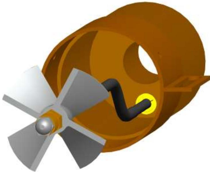
*Figure 25-25. Location of the Stator on the Fuel Tube*
