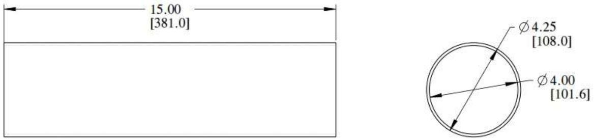
Figure 25-14. Dimensioned Drawing of the Draft Tube
