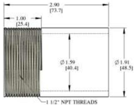
Figure 25-18. Dimensioned Drawing of the Pipe Nipple
