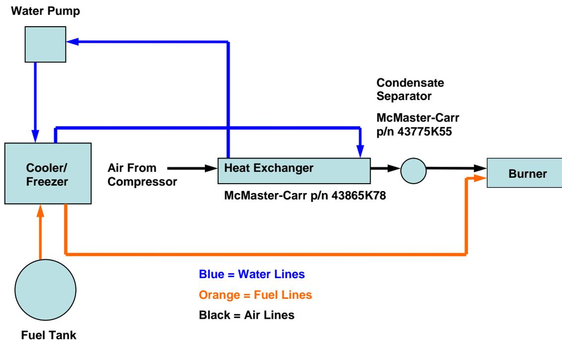
Figure 25-33. Schematic of Air/Fuel Heat Exchange System
