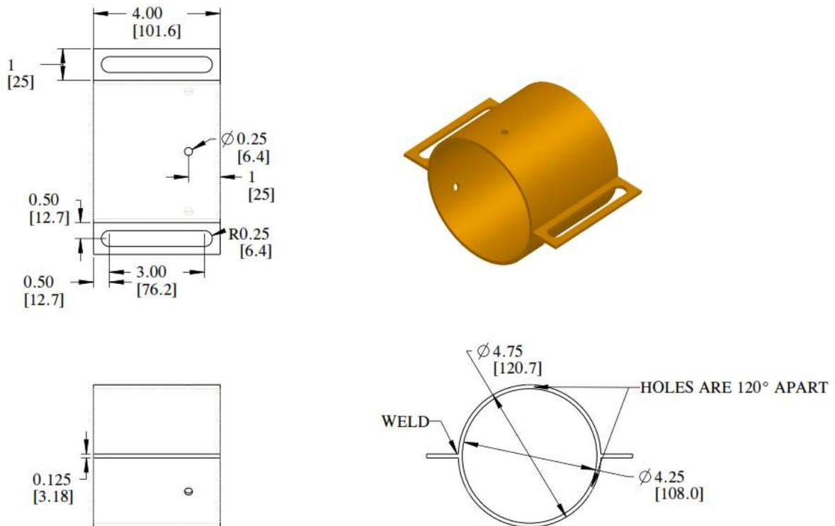
Figure 25-15. Dimensioned Drawing of the Coupling
