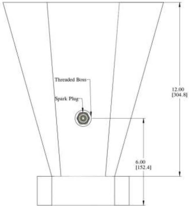
*Figure 25-10. Spark Plug Location in Burner Cone*
