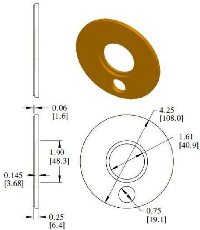
Figure 25-17. Dimensioned Drawing of the Back Plate
