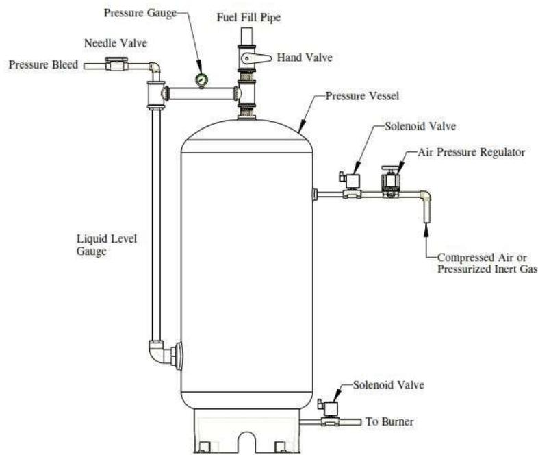
Figure 25-28. Schematic of Pressurized Fuel Tank System
