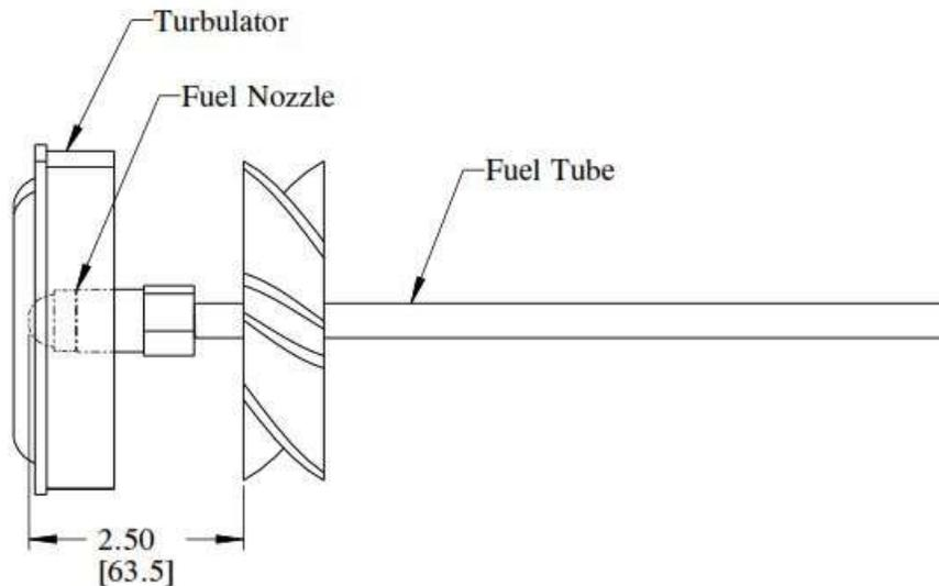
Figure 25-27. Typical Configuration of the Stator and Turbulator
