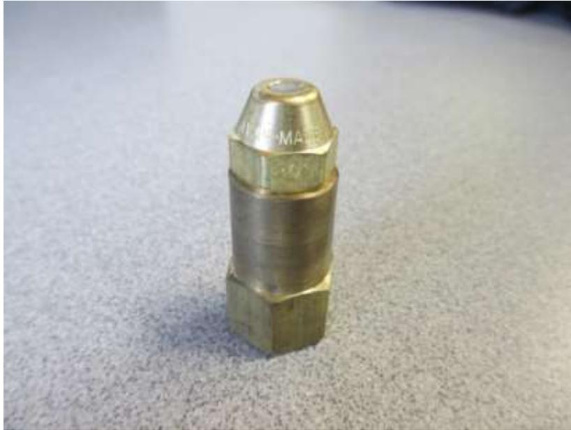
*Figure 25-31. Fuel Nozzle and Brass Adapter*
