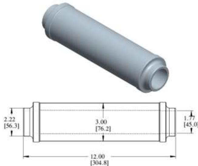
Figure 25-22. Schematic of the Muffler
