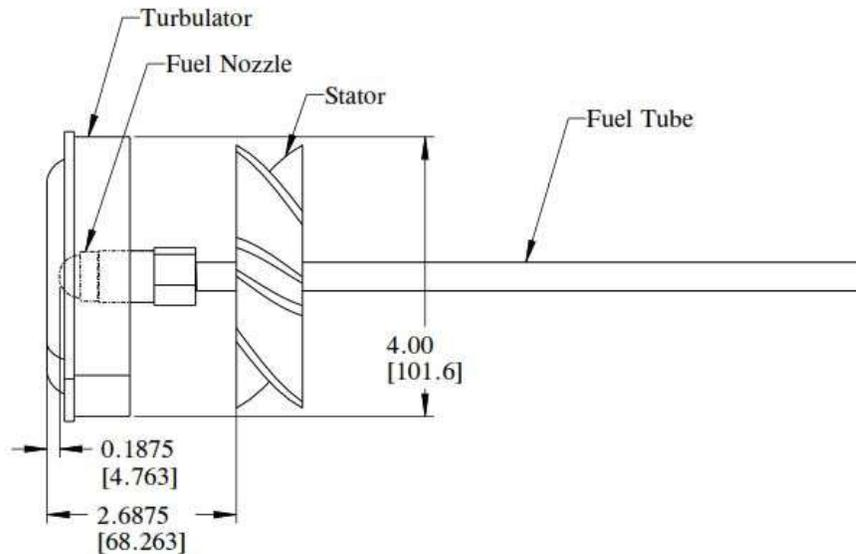
Figure 25-8 Fuel Nozzle and Stator Locations
