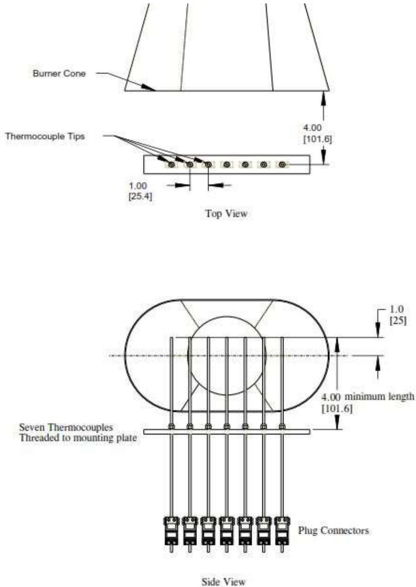
Figure 25-6. Top and Side View of Thermocouple Rake Bracket
