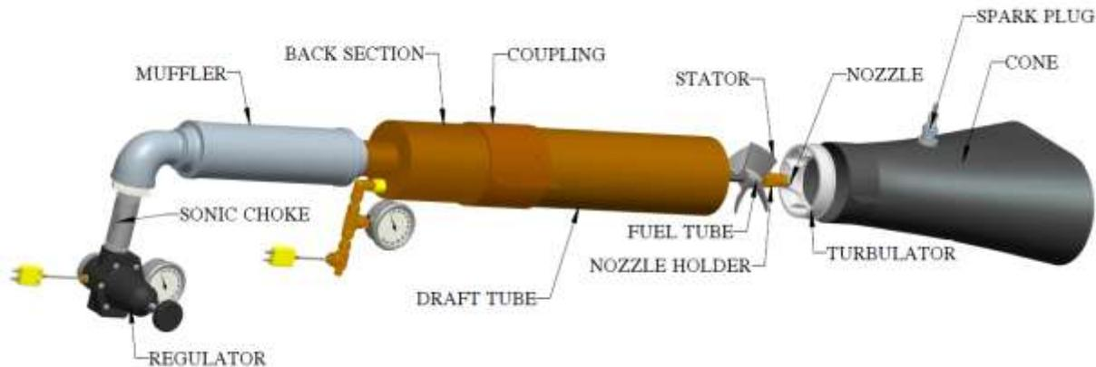
Figure 25-13. Schematic of the NexGen Burner - Exploded View
