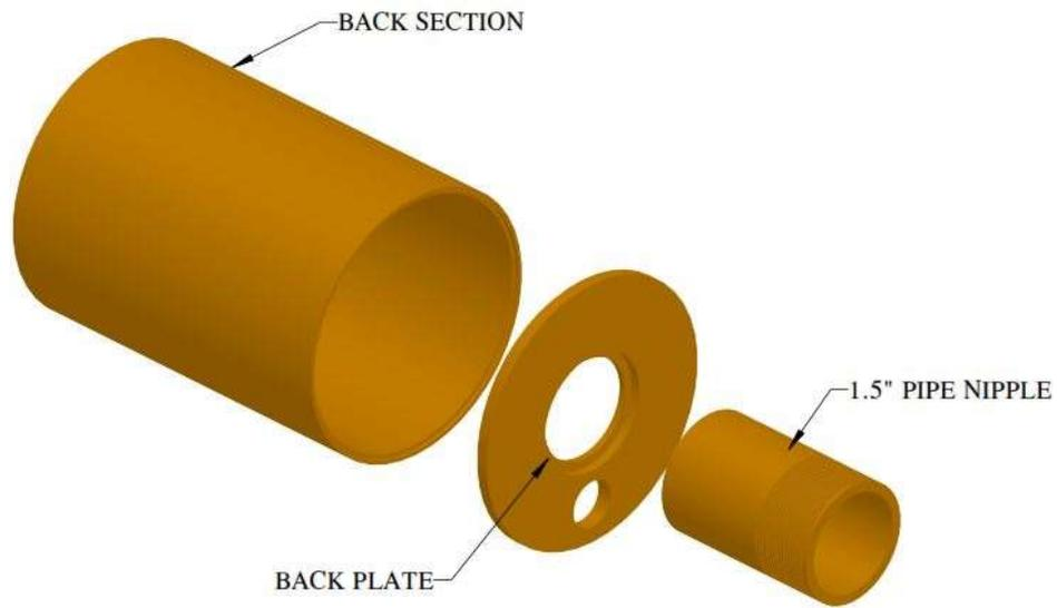
Figure 25-16. Back Section Components - Exploded View
