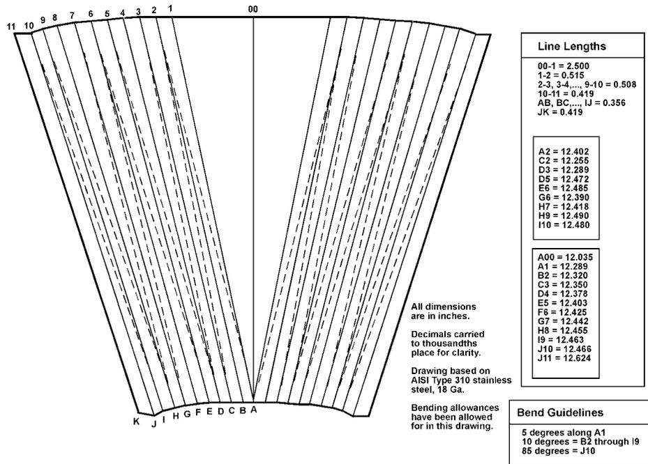
Figure 25-34. Burner Cone Layout and Bending Pattern
