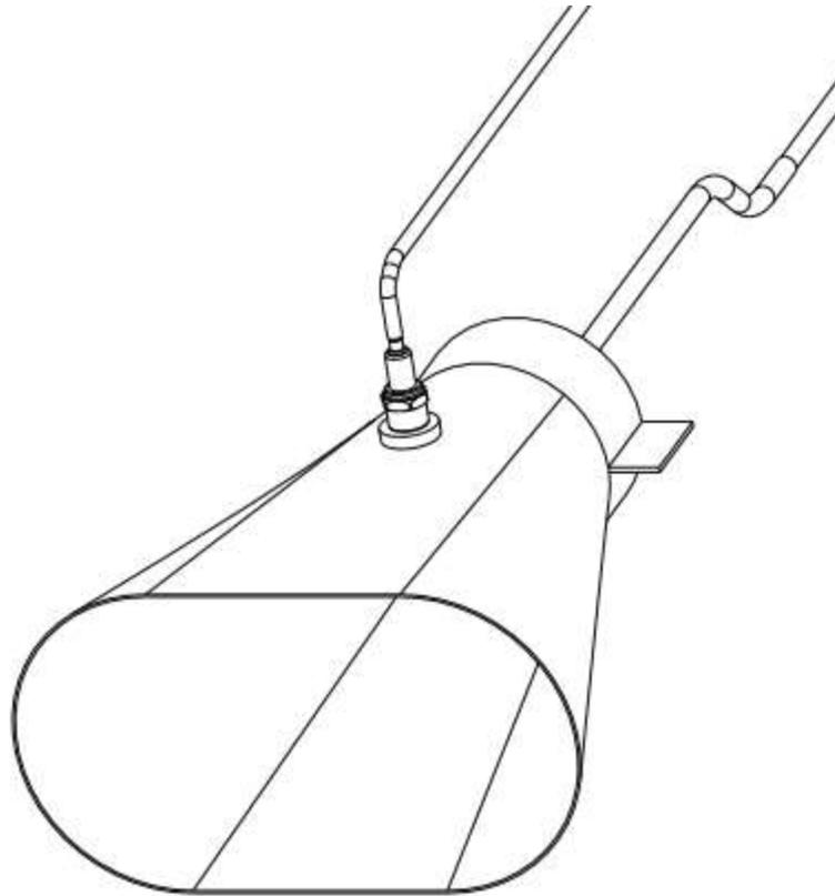
25-12. Proper Routing of the Spark Plug Wire
