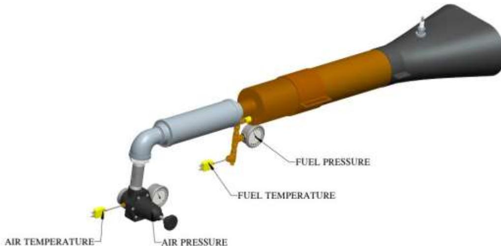
Figure 25-37. Burner Schematic Showing Inlet Measurement Locations
