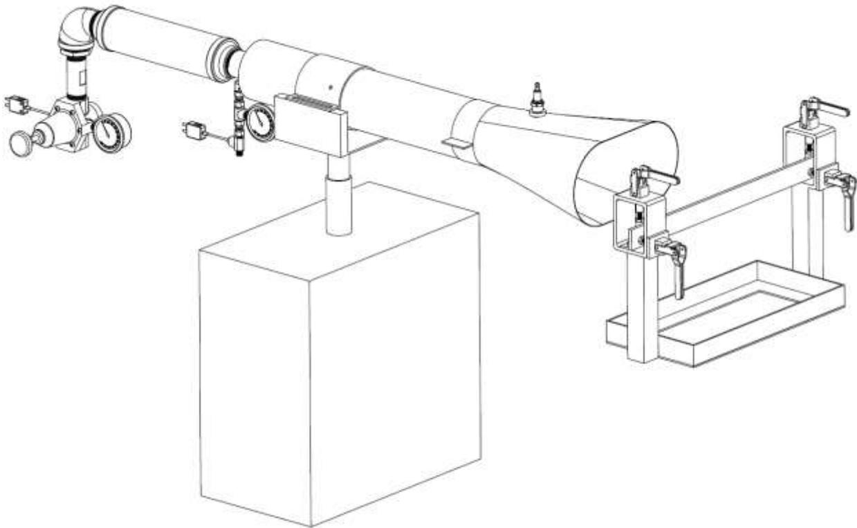
*Figure 25-1. Magnesium Alloy Testing Apparatus*
