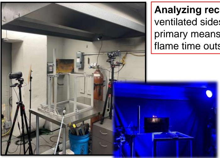
Analyzing recorded test videos of all ventilated sides of the enclosure is the primary means of defining the cumulative flame time outside of the enclosure
