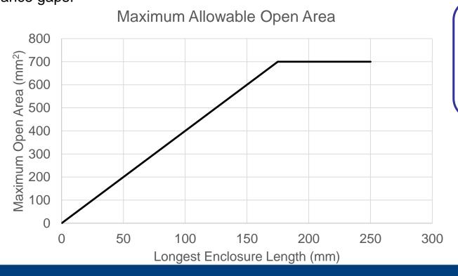
Only consider open area of the unit in its installed state.
