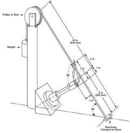
Figure 4-1. 60-Degree Electrical Wire Bunsen Burner Test Setup
