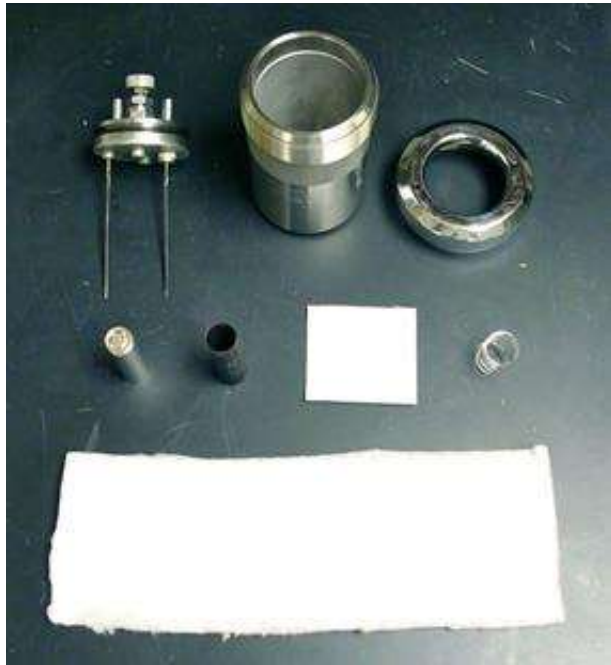
Bomb and other components for 18650 battery tests
