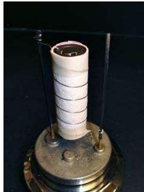
Bomb and other components for 18650 battery tests
