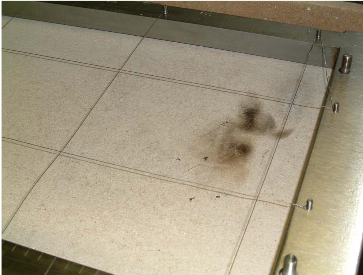
Restraining Wires Added to Frame
