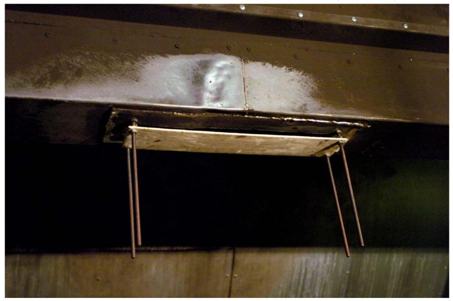
Intumescent Coated Steel Baffle 30 Seconds
