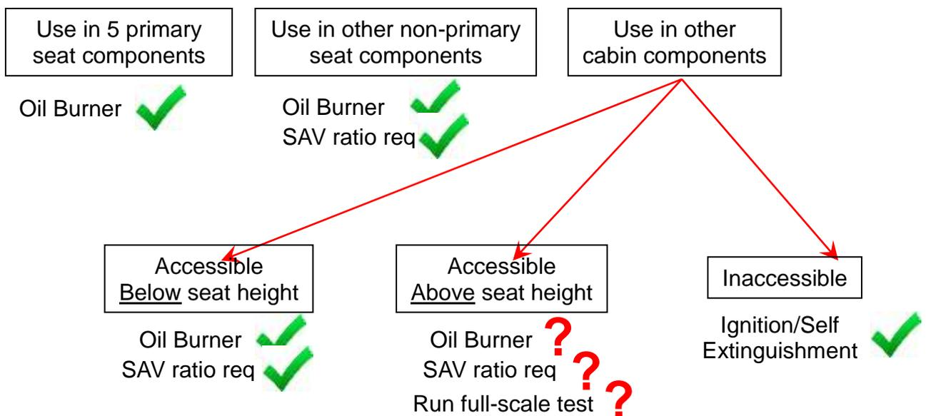
The FAA suggested that accessible, non-seat components located at or below 60 inches in height could also be substantiated using the maximum allowable SAV ratios
