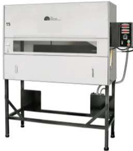
Radiant Panel (Thermo-acoustic Insulation) • Flame propagation distance • After flame time
