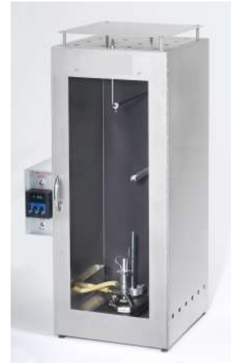
Vertical Bunsen Burner (All other materials) • Flame time • Flame drip time • Burn length
