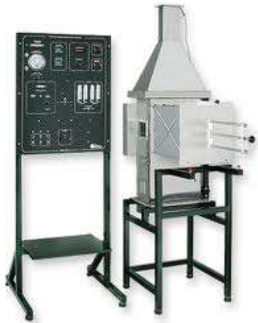
OSU Rate of Heat Release Apparatus (Large Area Materials) • Peak HRR • 2-min HR
