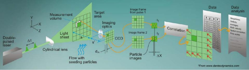
Particle Image Velocimetry (PIV) is a whole-flow-field visualization technique that provides instantaneous velocity vector measurements in a cross-section of a flow
