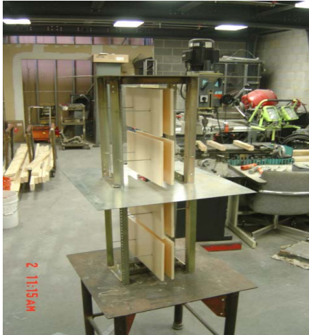
FIRST IDEA FOR COMPLEX GEOMETRY FIRE TEST SETUP
