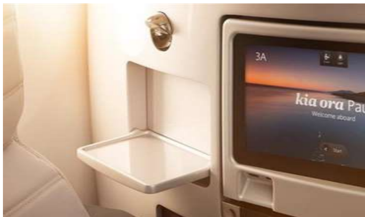
Figure1. Fold Down Cocktail Tray Produced with Additive Manufacturing
