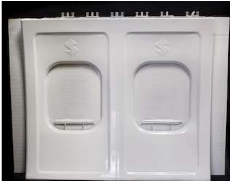
Figure 3. AM-manufactured cabin sidewall panel from Ultem 9085.
