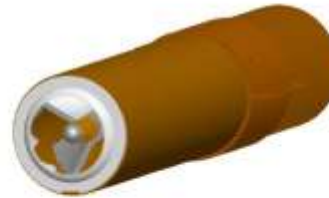
Figure 7-5-16. Position of Turbulator at the end of the Draft Tube
