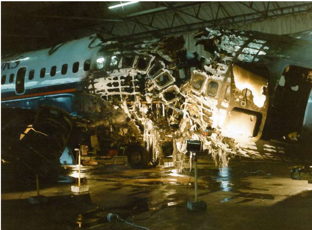
External Fire Damage: Left side aft of wing
