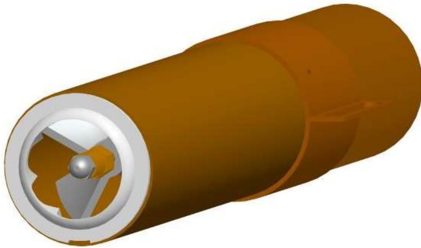
Figure 13. Position of Turbulator at the end of the Draft Tube
