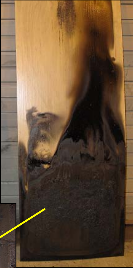
Premium structural fiberglass (FRP) severe black smoke up to 6 minutes after foam block ignition
