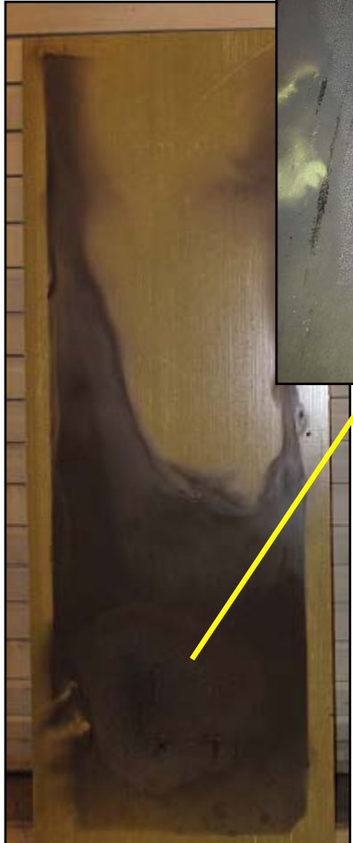
Structural fiberglass (FRP) no activity after foam block subsided
