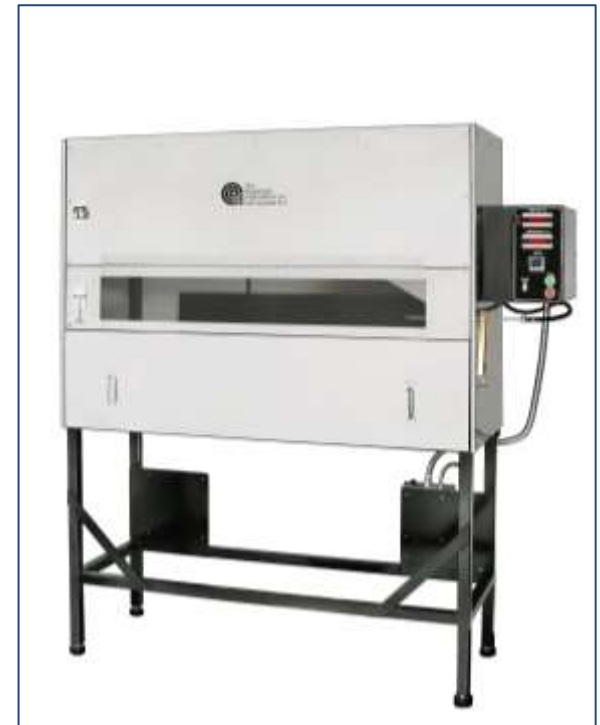
Radiant Panel (Thermal-acoustic Insulation)
