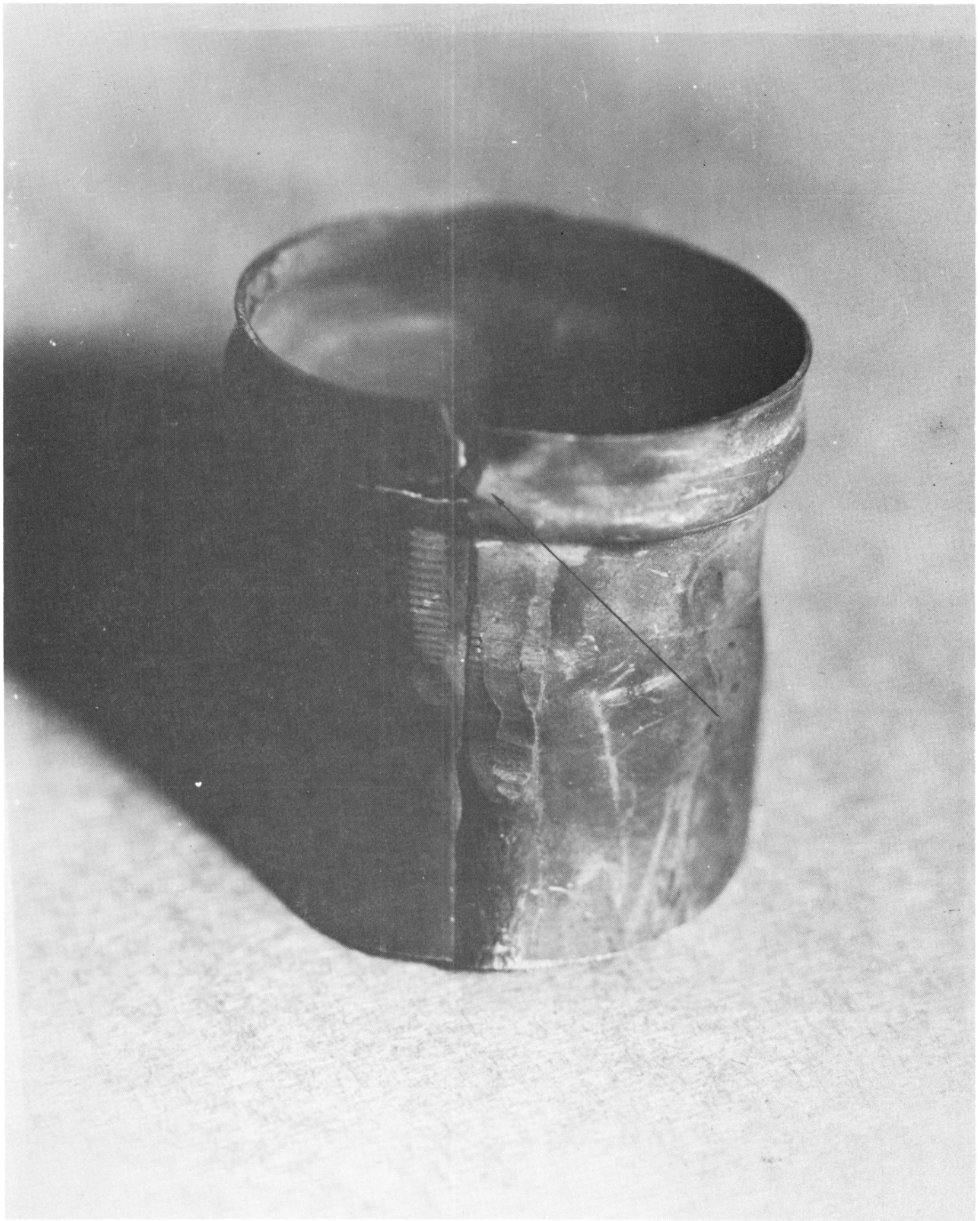
Figure 30. Sample No. 8 - Stack Joint, 112 Test Hours
