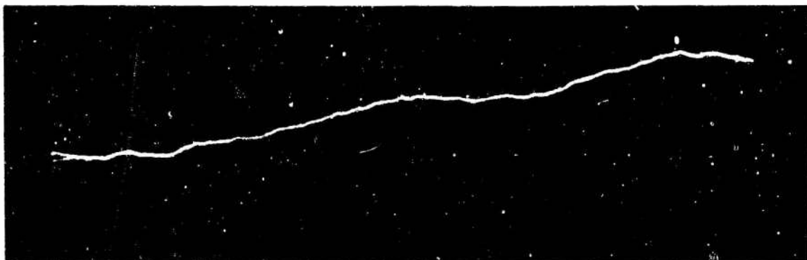
FIG. 2. Still photograph of a 4-m air spark between a positive rod and a negative plane.
