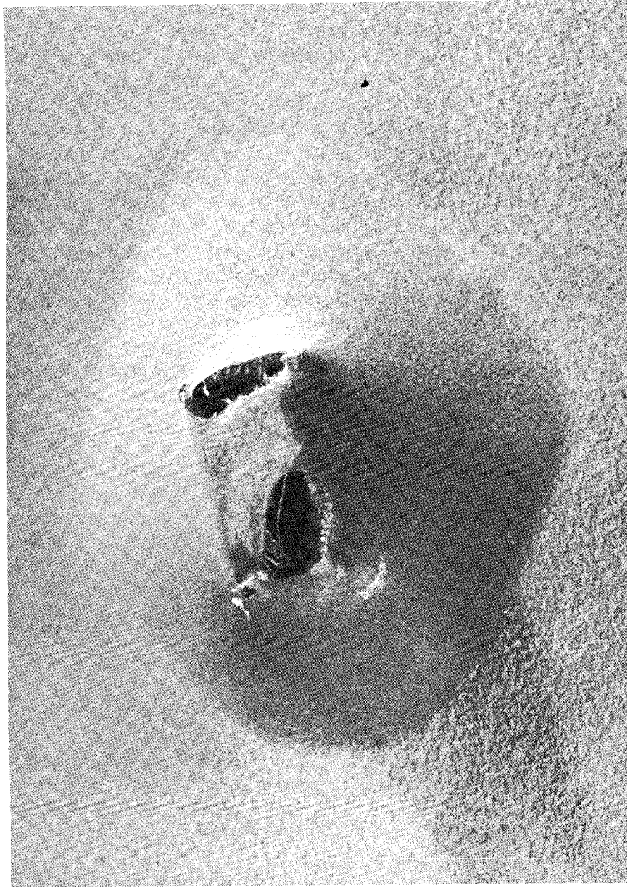
FIGURE 8 - INTEGRAL TANK LINER BONDED TO SIMULATED TANK WALL
